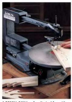
A SCROLL SAW is a favorite tool for cutting intricate curves and patterns. They are not powerful but are relatively easy to manage.
