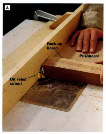
PHOTO A: Chamfer the top edges of each leg. A backup block of scrap wood prevents tear-out on the tralling edge of the cut, while a pushboard keeps it tight against the workpiece and permits a uniform, safe pass over the cutter and against the fence. Use a wood fence with a bit relief cutout.
