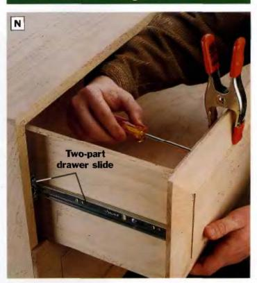
PHOTO N: Attach the drawer fronts to the drawers with screws driven through the front, inside face of the drawer box and into the back face of the raised-panel drawer front. Hang the drawer boxes first so the drawer fronts will be perfectly positioned.
