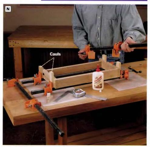
PHOTO N: Glue up the drawers, offsetting the cauis to allow the finger joints to close tightly. Clamp the finger joints from both directions, and measure the diagonals from corner to corner to check for squareness.
