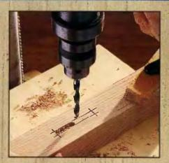
1 Carefully lay out your mortise using a marking gauge or straightedge.
