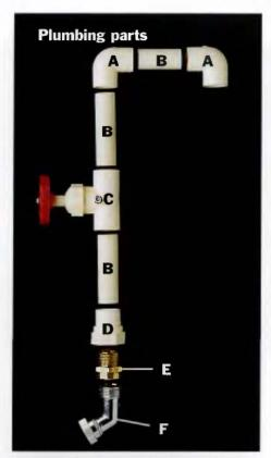
This plumbing system is designed to hook up to a garden hose for a water supply. To build it, you'll need: (A) 90° elbow; (B) 3/4-In. PVC pipe; (C) PVC stop valve; (D) Female adaptor; (E) Hose thread to pipe thread transition fitting; (F) Angled hose connector.
