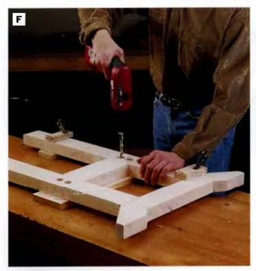
PHOTO F: Drill counterbore holes for the lag screw heads and washers, and drlll clearance holes and pilot holes for the shanks of the screws.
