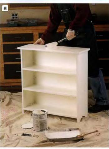
PHOTO H: Roll or brush on a coat of primer to all exposed surfaces, followed by two coats of paint.
