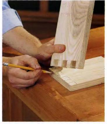
Once the pins are cut, lay out the tails by laying the pin board on the face of the tail board and marking the pin profiles. Use a sharp pencil so the marks are true. Also use a marking gauge to scribe a line on the face of the board, establishing the bottom line for the tails. Make sure the pin board and tail board are flush at the edges before making any marks.
