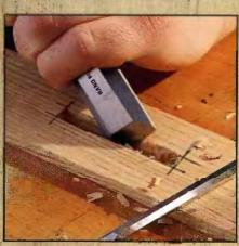
2 Use a sharp chisel to clean up the sides of the mortise so they're flat and smooth. Make sure the flat face of the chisel is contacting the wood. Clean up the ends of the mortise with a chisel the same width as the thickness of the mortise.
