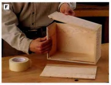
PHOTO F: Apply glue to the mitered faces and use tape to hold the corner joints together while the glue sets. Tack the box bottom panel into Its rabbet. The IId panel dado gets no glue.
