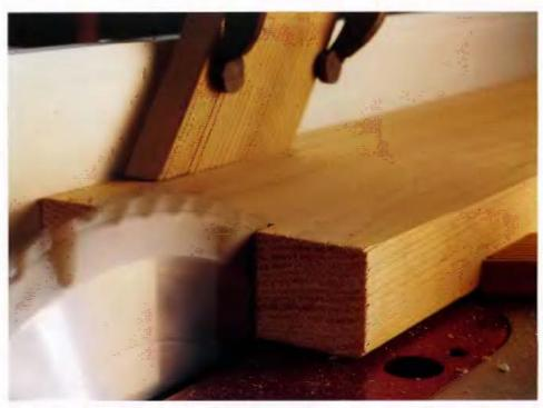
Ripping boards to width should be done after one edge has been squared (see previous section) so a fiat even surface can ride against the saw fence or be used to register your straightedge for making rip cuts with hand-heid tools.
