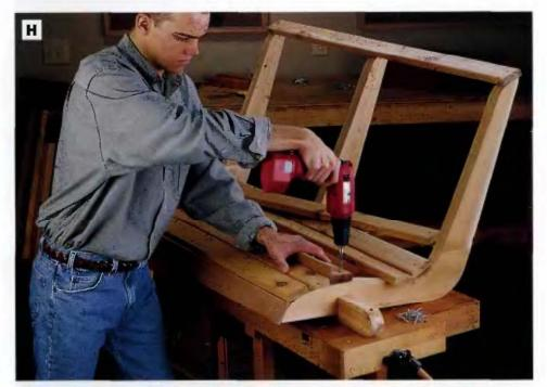
PHOTO H: Screw the slats to the back-and-seat support structures. Butt the first three slats together, then use a ¼-in.-thick spacer between the rest of the slats for consistent gaps. Keep the ends of the slats flush with the sldes of the supports.
