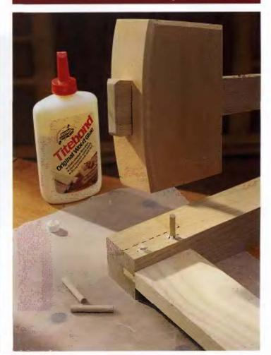
Cut the pins from hardwood doweis, normally of the same species as the workpieces. Tip: For a decorative touch, use doweis made of wood with a naturally contrasting wood tone (for example, maple pins driven into wainut workpieces). Taper the lead tip of the dowei slightly so it will enter the hole more easily. Squeeze a little glue into each hole, then tap the dowel pins home with a wood mailet. Stop tapping when the dowel seats at the bottom of the hole.
