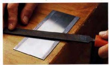
File down any traces of the old burrs on all edges of the cabinet scraper, using a fine single-cut metal file. Don't get too aggressive with the file—it doesn't take much power to remove a fine burr.
