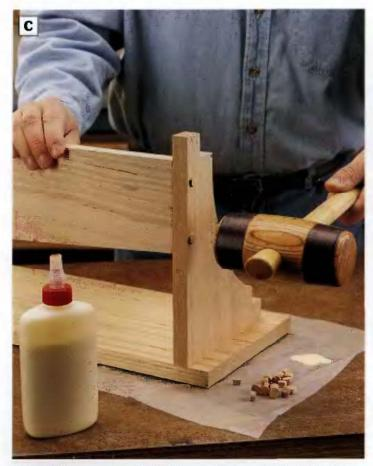
PHOTO C: Once you've attached the coatrack parts, cover the screwheads with face-grain red oak piugs heid in piace with giue. Tap each piug into its counterbore with a wooden maiiet.
