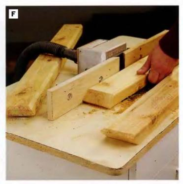
PHOTO F: The bottom edge and both ends of each apron plece are chamfered. Make these cuts at the router table, using a plloted chamfering bit set to a height of  $^{3}/8$  In.
