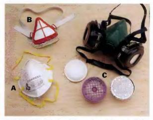
PROTECT against dust and fumes. A particle mask (A) is a disposable item to be worn when doing general shop work. A dust mask (B) has replaceable filters and flexible faceplece to keep out finer particles, like sawdust and insulation fibers. A respirator (C) can be fitted with filters and cartridges to protect against fumes and very fine particles, especially when working with chemicals.
