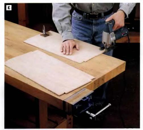
PHOTO E: Using a jig saw, notch out the corners of the chest bottoms so they will fit around the ungrooved side stiles.
