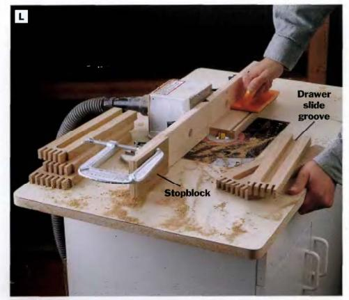
PHOTO L: After the drawer bottom grooves have been cut on the router table, rout grooves for the drawer sildes. Both are stopped dadoes, cut in multiple passes.
