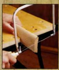
With the square-cut board flush Lin the corner, use a coping saw to trim the excess wood from the beveled end, leaving an end that's perpendicular but tapers up to foilow the profile of the molding.
