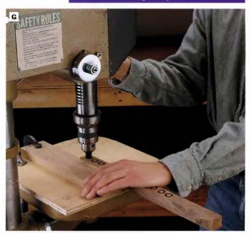
PHOTO G: Make wainut screw plugs on the drill press, using a 38-in. tapered plug cutter. Clamp a scrap piece to the drill press table to create a surface that helps keep the wainut stock stationary while you cut the plugs.
