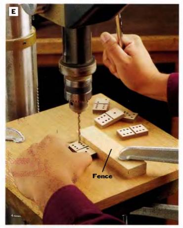
PHOTO E: Driii shailow holes through the maple veneer and just into the wainut core to create the domino dots. Set the depth stop to keep the bit from driiiing too deeply. Clamp a fence to the driii press table so the rows of dots will line up lengthwise along the dominoes. Work carefully when driiling to hit your dot locations precisely.
