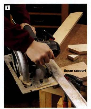
PHOTO I: Mark the angled ends of the runners and cut the corners with a circular saw. Support your straightedge from beneath with a wood scrap ciamped to the workbench.
