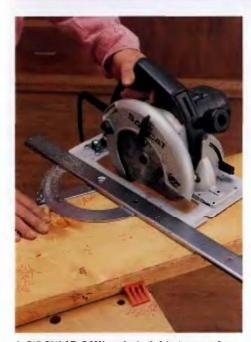
A CIRCULAR SAW and straightedge cutting guide can be used for cross cuts, rip cuts, bevel cuts and miter cuts.
