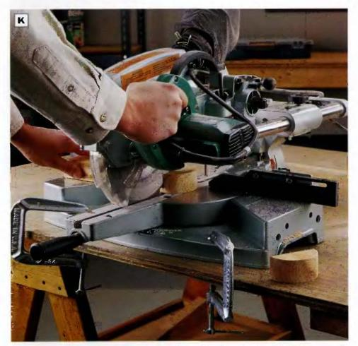
PHOTO K: Cut  $1^3$ /4-in. radiuses on either end of a section of  $2 \times 4$  cedar. Cut off these curved ends with a power miter saw or radial-arm saw. The pieces will serve as leg stops on the foot rest. Cutting short workpieces from longer stock keeps your hands a safe distance from the blade.
