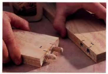
After drilling all the holes, apply a dab of glue into each hole. Also apply glue to the mating wood surfaces. Silde the dowels into the holes to make the joint.
