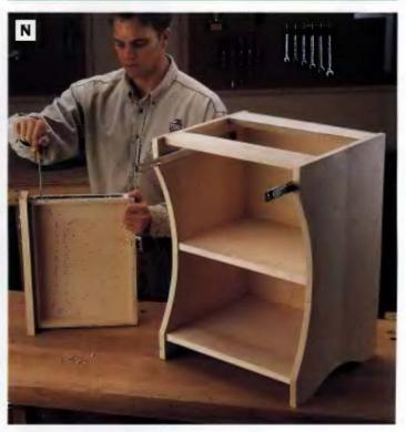
PHOTO N: install the full-extension metal drawer slides and hang the drawer in the cabinet carcase. Be sure there is an even overhang between the drawer face and the cabinet carcase.
