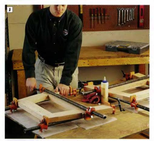
PHOTO J: Build the glider stand ends by attaching the top and bottom end rails to the stand iegs with doweis and glue. The bottom rails fit between the iegs, while the rop rails overlap the top ends of the legs.
