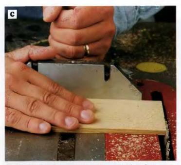
PHOTO C: Tit the table saw blade to 13° and bevel-cut the top and bottom ends of the stand biank. Hold the workpiece against the miter gauge to make these cuts.
