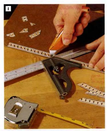
PHOTO I: Miter-cut the corners of the decorative iniay strips using the 45° fence on a combination square and a sharp utility knife. Hold the knife as square to the iniay as you can when making the cuts, so the mitered joints will meet flush.
