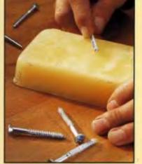
Keep a block of beeswax in your shop to lubricate the threads of screws. The wax greatly reduces friction, which makes for less work and fewer stripped screw heads. You can use hand soap for a similar purpose, but it's more likely to discolor the wood.
