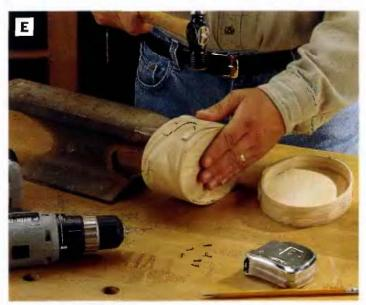
PHOTO E: Drill pllot holes through the fingers on the Ild and box sldes, then tap the decorative brass pins into the pilot holes and against an anvil to flatten and bend over the pln tlps inside the box.
