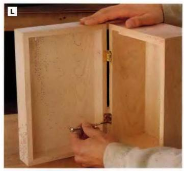
PHOTO L: Measure and cut the hinge mortises with a wood chisei, then install the brass jewelry box hinges to attach the iid to the box.
