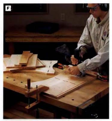
PHOTO F: Cut biscuit slots in the sldes and In the ends of the bottom, top stretchers, and shelf for assembling the carcase. Clamp a plywood straightedge to the slde panels to help align the base of the biscuit joiner when cutting blscuit slots In the slde panels.
