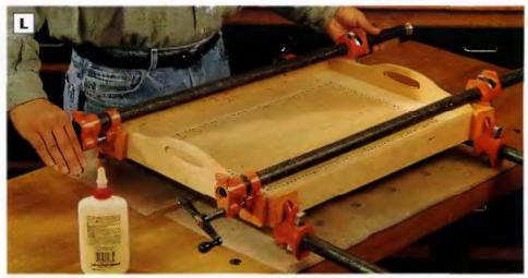
PHOTO L: Spread giue onto mating surfaces of the finger joints, siip the bottom into its grooves and clamp up the tray. instail clamps both lengthwise and widthwise to hold the finger joints closed in two directions.
