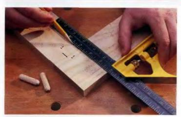
To lay out the dowel joints, but the two mating parts together, making sure the mating surfaces are flush. Mark the dowel hole locations by drawing a single line across the joint for each dowel. For best results, use at least two evenly spaced dowels at each joint.
