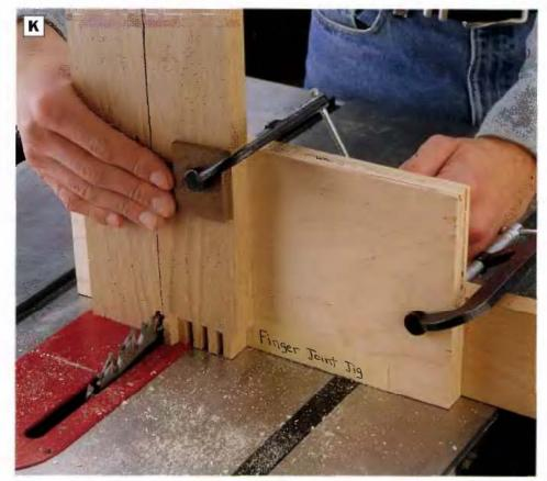
PHOTO K: For boards that start with a slot, not a pin, use the mating board as a guide for cutting the initial slot. The end slot on the cut board fits over the pin spacer strip, with the outer pin on the workpiece fitting between the strip and the saw blade.
