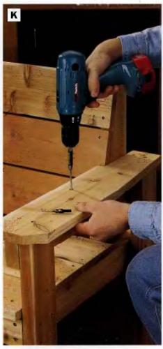
PHOTO K: Position the arms on the leg assemblles and fasten them to the arm supports and the legs with screws.
