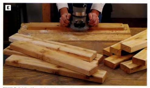
PHOTO E: Cut the 19 seat slats to length, and ease the top edges and ends of each slat with a ½-in. roundover bit in the router. We used a plywood jlg clamped to the benchtop to "frame" each slat on all sides and hold it steady while routing. This way, the slats require no further clamping.
