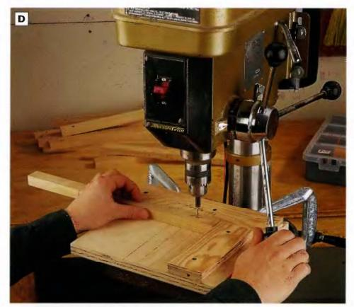
PHOTO D: Build a right-angle jlg from scrap to help index placement of the counterbored holes In the ends of the slats. Clamp the jig to the drill press table so each slat is exactly aligned for drilling when you lay it in the jig. This way, there's no need to measure and mark each siat hole.
