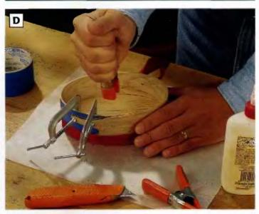
PHOTO D: Glue the side pieces to the box top and bottom. Hold the bentwood parts in position while the glue dries with strap, spring and C-clamps. Mask off the area around the fingers to protect these spots from glue squeeze-out.
