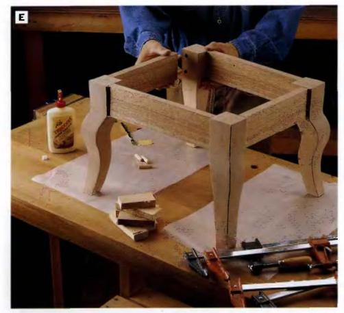
PHOTO E: Glue the dowel joints, insert the dowels and assemble the base. Clamp across the sides with bar or pipe clamps. Measure across the corners of the assembly and square it up.
