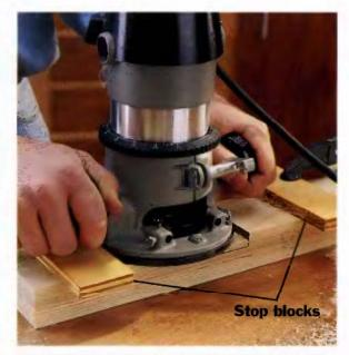
USE A ROUTER. Mount a straight bit in your router and set the cutting depth to equal the depth of the notch. Ciamp stop block guides to the workpiece at each end of the notch. The guides should be positioned so their distance from the end cutting lines is the same as the router setback (the distance from the bit to the edge of the base). Remove the waste wood with the router, working between the stop blocks (the central area of the notch is routed freehand).
