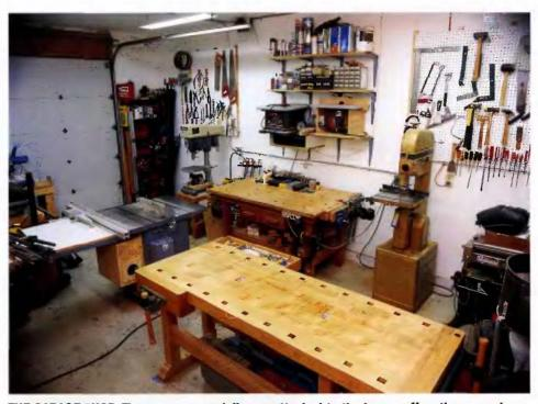
THE GARAGE SHOP: The garage, especially one attached to the house, offers the convenience of a basement shop with fewer drawbacks. Overhead doors provide excellent access, greater headroom, lower humldity and better ventilation. The main general drawback is that garages are usually home to one or more vehicles and a host of other outdoor items. A good solution is to mount your stationary tools on casters so they can be wheeled out of the way to make room for other things.
