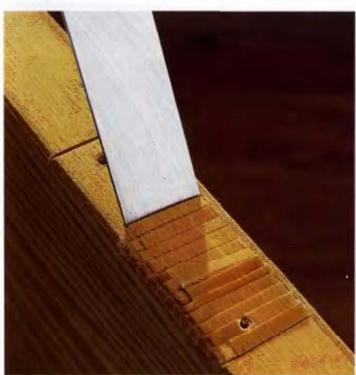
With the beveled edge of the chisel tip flat against the workpiece, make a series of rellef cuts in the waste wood area of the mortise. Space the cuts ½ to ¼ in. apart (make closer cuts in harder woods). The cuts should be equal in depth to the finished depth of the mortise.
