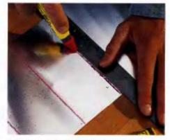
USE A GREASE PENCIL to mark metal, plastic and other materials that can't be marked clearly with a pencii.
