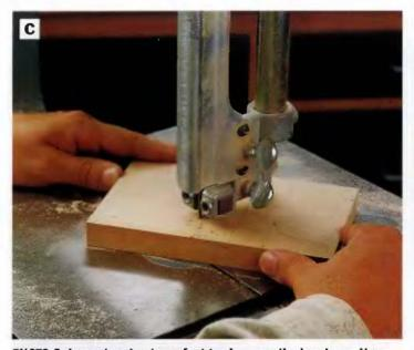
PHOTO C: Lay out and cut one foot to shape on the band saw. Use this workplece as a template for drawing and cutting the second leg to shape. Then clamp the legs together and sand both smooth at one time.
