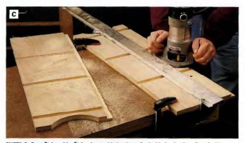
PHOTO C: Rout ¾-in.-wide, ¾-in.-deep rabbets along the inside back edge of each side panel for the bookcase back. Clamp each side panel to your bench to hold it securely as you rout the rabbet, and guide the router base against a straightedge.
