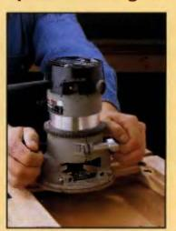
USE A PILOTED RABBET BIT to cut rabbets on the insides of frames or on the outer edges of any workpieces. Make several passes of increasing depth with the router, then square the rabbet corners with a chisel. When profiling an outside edge, clamp scrap blocks at the ends of the workpiece.
