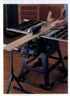
A TABLE SAW is the most heavily used tool in most woodshops. It can make just about any straight cut, including beveis and miters.
