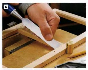
PHOTO C: Square off the inside chamfered corners of the face frame with a chisel. Lay out these corners first with a pencil and square, then pare up to your layout lines.
