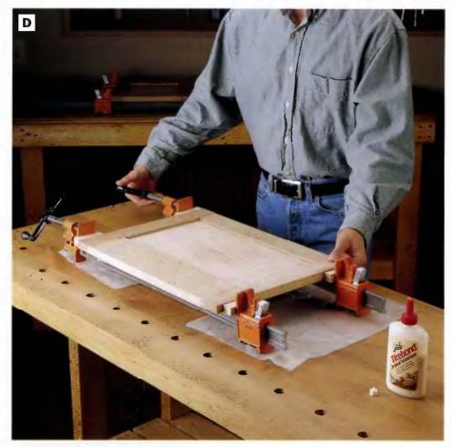
PHOTO D: Giue and ciamp up the frame-and-panel assemblies for the back and the sides. Make sure the ends of the stiles are flush with the edges of the rails. Do not glue in the panels-they should "float" in the grooves.
