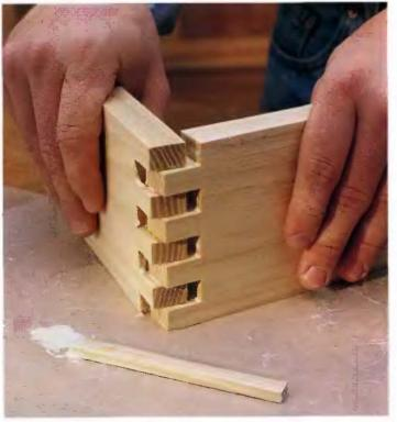
**6**When ail the joints are cut, the pieces are ready for assembly. Give the joints and clamp them together with wood cauls offset from the joints to allow the joints to close.
