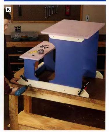
PHOTO K: Fasten the runners to the bench and desk legs with countersunk 11/4-in. drywaii screws. Hold the parts together with clamps while you drive the screws. Stagger the screw pattern.
