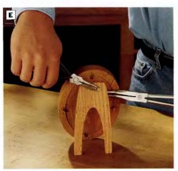
PHOTO E: After locating the hinge position, mount the hinge to the frame back with #4 imes imes imes imes flathead wood screws. Fasten the hinge to the stand with bolts and nuts. Arrange the bolts so you can thread the nuts on from the back of the stand. Tighten the nuts and bolts with a pair of needle-nose pilers.
