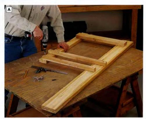
PHOTO A: Build the right assembly by attaching a drawer stretcher, drawer slide and lower stretcher between a tall leg and front leg. Fasten the parts together with 2½-in. deck screws. Use a combination square to draw layout lines for the parts and to check the joints for square.
