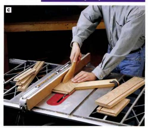
PHOTO C: Cut  $44 \times 36$ -in. grooves for the upper and lower chest bottoms into the side and front rails. Use a featherboard and pushstick.
