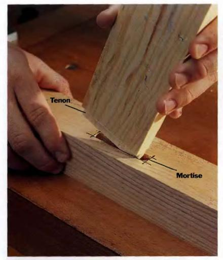
THE MORTISE-AND-TENON is one of the simplest and strongest wood joints. It's comprised of a narrow tenon carved in the end of one mating workpiece, which fits into a mortise hole in the other mating workpiece. The joint can simply be glued, or you can reinforce it with dowels or wedges.
