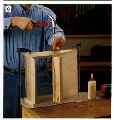
PHOTO C: Giue and nail the sides to the bottom and cookbook rest to form the recipe box. Arrange and clamp the parts so you can nail through one side, then reciamp and fasten the other side.
