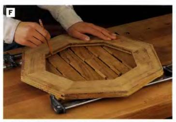
PHOTO F: Insert ¼-in. spacers between the slats and clamp them together. Lay the rail assembly over the slats and trace the interior of the assembly onto the slats.
