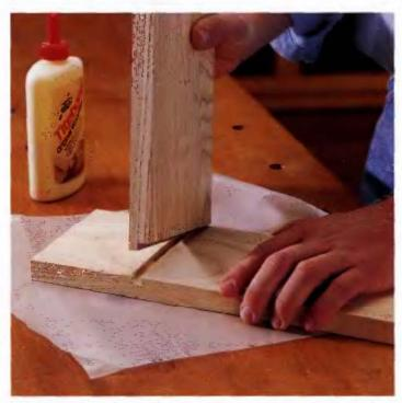
TEST-FIT THE JOINT and adjust the thickness of the rabbet ledge by trimmling, if needed. Apply glue to both surfaces, then assemble and clamp the joint.
