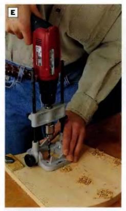
PHOTO E: Drill 1/2-in-deep dowel holes at the dowel hole centers you marked on each of the two sides with the hardboard template.
