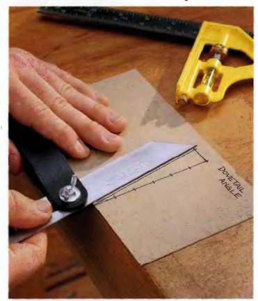
1 Draw the dovetall pin angle and use it to set the angle on a sliding T-bevel that you can use to mark the pins on the ends of the pin boards. Make a scale drawing of a dovetail pin and use it to set a sliding T-bevel for marking the layout lines for the pins. A standard angle is 80°, which equals a 1:6 ratio of slope to pin depth.
