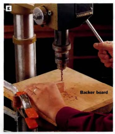
PHOTO E: Bore ¼-in.-dla. holes for the perches through both ends of the base strips. We stacked these parts and drilled both strips at once on the drlll press.
