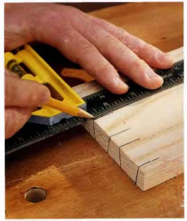
Finally, transfer the lines drawn on the end of the board to both faces of the board with a try square or combination square.
