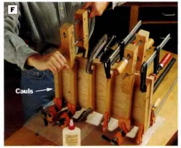
PHOTO F: Laminate two ¼-ln. plywood sheets together to form the bottom panel. Ciamp up the piywood on both sides with iong wood cauls to press the sheets tightly together until the glue dries.
