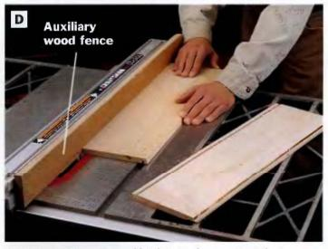
PHOTO D: Cut the bottom rabbet into the lower edge of the box sides. Attach an auxiliary wood fence If you use a table saw and dado-blade set to cut these rabbets.
