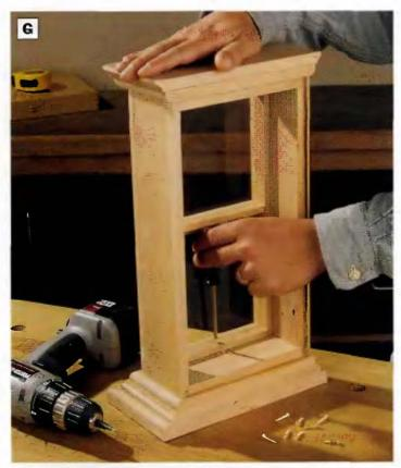
PHOTO G: Install the glass and retainer frame with a pair of brass wood screws—one through the retainer top rall and one through the bottom rail. Countersink these screws.
