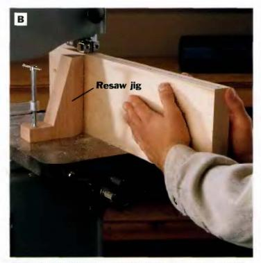
PHOTO B: Resaw the maple stock in half for the sides and ends of the box, using a marked centerline as a gulde for the blade. A shopmade resaw jig clamped to the saw table will help square the board to the table and keep the blade tracking along the cutting line.
