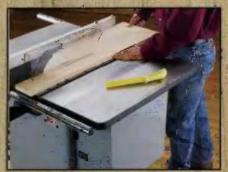
1 Start rip cuts with your left foot against the front left corner of the saw base. Feed the workpiece with your right hand, and use your left hand to keep the workpiece snug against the rip fence. Use a pushstick whenever a workpiece requires your hand to be closer than 6 in. to the blade.
