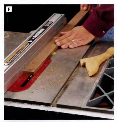
PHOTO F: Cut the ¼-in-wide groove for the box bottom using a dado biade in the table saw. Then install a ½-in.-kerfed blade in the saw and cut a groove for the sliding iid along the opposite long edge of the workpiece. Cutting these grooves now allows you to work more safely with a long workpiece and ensures that the grooves will align perfectly when you assemble the box later.
