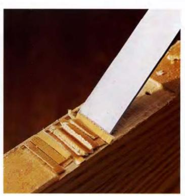
Clean out the waste wood by driving the chisel against the direction of the relief cuts. To avoid digging in too deep, try to keep the beveled edge of the tip flat in the mortise. Scrape the bottom of the mortise smooth. If you need to deepen the mortise, repeat the procedure—don't simply try to make deeper scraping cuts.
