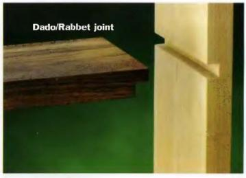
style features a rabbet with a tongue half the thickness of the workpiece that fits into a matching dado or groove. This joint is used commonly to fasten shelves to upright standards, such as bookcases. The ends of the shelves receive the rabbets, while the standards are dadoed. Another less com-
