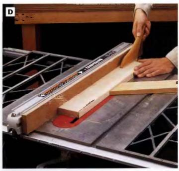
PHOTO D: Resaw 1/8-in.-thlck edging strips from 4/4 maple stock, using a table saw or band saw. Joint the cut edge of the board flat before you rip each edging strlp.
