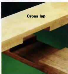
LAP JOINTS are, in essence, extra-wide rabbet and dado joints. They're used primarily in furnituremaking and frame-making, where the extra gluing surface in the sturdy interlocking joints greatly increases the strength of any project.
