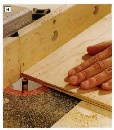
PHOTO H: Rout a shailow rabbet around the top face of the bottom panel for the veneer inlay strips. Install a ½-in. straight bit in your router table to cut this ½2-in.-deep rabbet. Practice on scraps first and test the fit of the strips in the rabbet.
