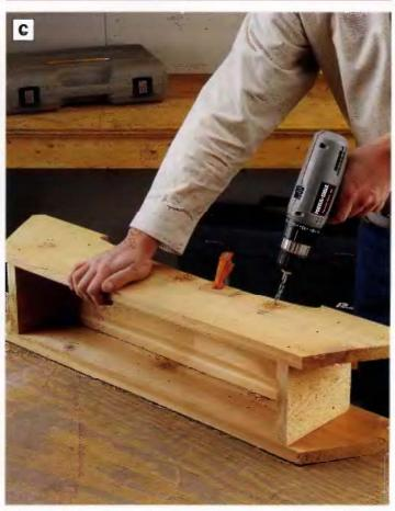
PHOTO C: Fasten the planter sides to the ends and bottom with nails, then drill three angled <sup>1</sup>/<sub>4</sub>-in.-dla. weep holes through the side where the bottom of the planter slopes to its lowest point.
