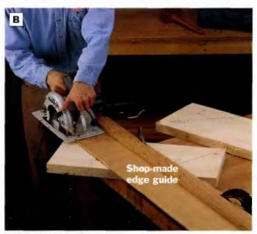
PHOTO B: Gang-cut the carcase top and bottom panels to size, then gang-cut the fixed shelves. Use an edge guide clamped to the work-piece and your workbench to ensure straight cuts.
