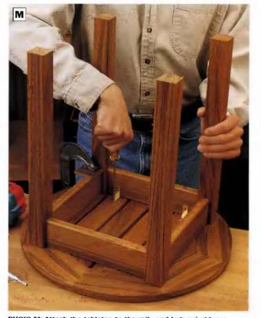
PHOTO M: Attach the tabletop to the rails and legs using brass L-brackets. Drlll pilot holes before drlving the screws.
