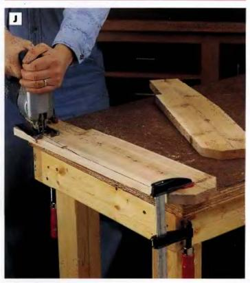
PHOTO J: Cut out the arms with a jlg saw, with the workpieces clamped to your workbench.
