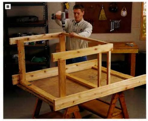
PHOTO B: Assemble the bench framework by attaching the two back stretchers, shelf stretcher and top front stretcher to the end assemblles. The ends of the stretchers should butt against the Inside faces of the front and back legs. See Step 4 for exact stretcher placement.
