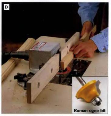
PHOTO D: Rout an ogee profile along one edge of both shelf edge strips with a plloted 5/32-In.-radlus Roman ogee blt (See inset). The edging is oversize at this stage to keep your fingers clear of the bit.
