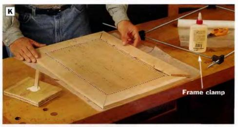
PHOTO K: Attach the frame sides and ends to the iniaid bottom panel with give and biscuits. Dry-fit the parts together first with the biscuits in place. Once the pieces are glued and fitted, install a frame ciamp around the assembly and tighten.
