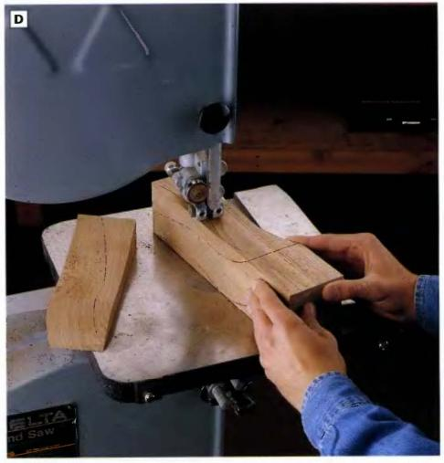
PHOTO D: Cut the profile on the adjacent side of each blank just as you did with the first side. The reattached waste pleces lend you flat surfaces for easier, accurate cuts.
