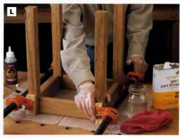
PHOTO L: Glue and clamp the legs and ralls together. Use clamp pads between the clamp jaws and mineral spirits to clean up squeeze-out.
