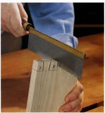
1 1 Ciamp the board in a vise and use a dovetail saw to make the cuts down to the scribed line. Remove the waste from between the tails with a sharp chisel, the same way you removed the waste from the pin boards. Make the shoulders of the tail board by sawing along the base line to the first tail on each end.
