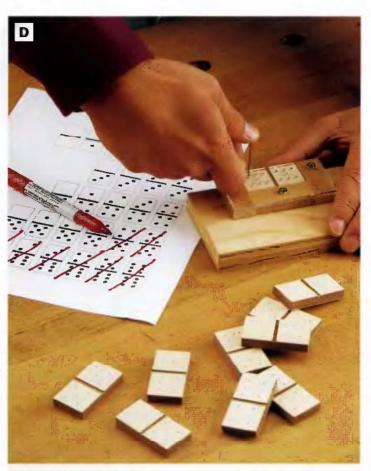
PHOTO D: Mark the dot iocations on the domino bianks, using the Tile Holes & Centerlines pattern drawing on page 289 as a guide. For greater precision, we built a simple jig with a clear Piexigias top drilled with ½16-in.-dia. holes at each dot location. We pressed a finish nail through the appropriate holes in the Piexiglas to mark each dot pattern.
