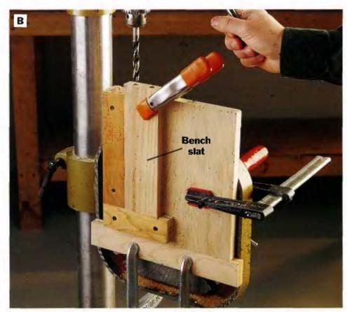
PHOTO B: A right-angle jig will make the job of drilling dowel hoies in the slats quicker and more precise. Tip the drill press table vertically and clamp the jig in place so the bit aligns with the dowel locations on each slat. Flip the slats edgewise and endwise to drill all four hoies.
