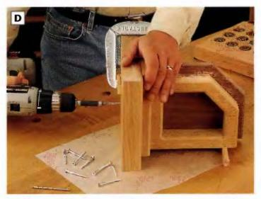
PHOTO D: Attach the bases to the frame/base cap subassembiles with glue and countersunk 2-in. wood screws. Clamp and fasten the parts together carefully to keep from spliling the ballast.
