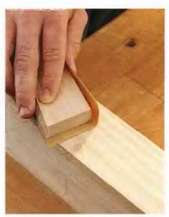
After the glue has dried, trim the plug flush with the wood surface using a flush-cutting saw (See photo, above left). Take care not to mar the surrounding wood surface. Sand the plug smooth.
