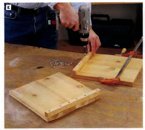
PHOTO E: Clamp pairs of 6-in.-wide boards for the end panels and fasten each panel together with a cleat. Use 1<sup>1</sup>/<sub>4</sub>-in. galvanized screws to join the parts. These two cleats are permanent parts of the planter.
