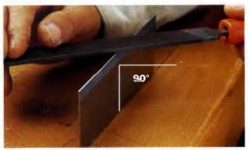
With the cabinet scraper held firmly in a vertical position, file the edges flat at an exact 90° angle, using the metal file. Take care not to overwork the edge.
