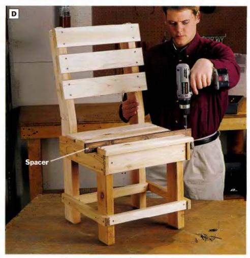
PHOTO D: To create uniform slat spacing, use a 1/2-in. spacer for positioning the seat slats and a 11/4-in. spacer for the back slats. Start the back slats at the bottom of the back leg angle. Install the seat slats so the back seat slat butts against the back legs.
