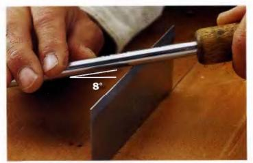
A Scrape across the edge of the scraper with the burnishing tooi, hoiding the tooi at an angle of about 8°. This will create a siight burn that accomplishes the cutting action of the scraper. Create burns on all four edges of the scraper, flipping the tool as each edge becomes duil.
