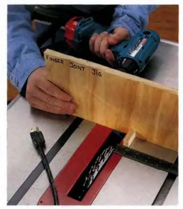
Reset the auxiliary fence by moving it a distance equal to the thickness of one pin to the outside edge of the biade set.
