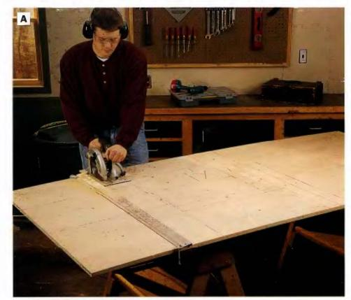
PHOTO A: Draw a cutting diagram on the piywood sheet to iay out the project parts. Mark each part with a letter that corresponds to the *Cutting List* on page 272 to help identify them. Clamp a straightedge in place to guide the saw as you cut the parts to size.
