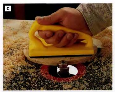
PHOTO C: Use a piloted rabbeting bit in the router table to mill the rabbet around the edges of the lid top. Hold the workplece securely against the router table and bit with a foam-soled pushpad. Feed the workplece around the bit clockwise to cut the rabbet.
