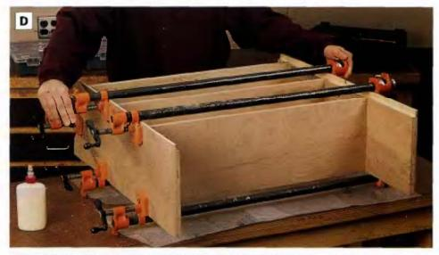
PHOTO D: Glue and clamp the shelves into their dadoes in the bookcase sides. Keep the shelves flush with the front edges of the sides so they don't obstruct the back rabbets.
