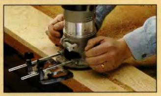
ROUTER EDGE GUIDE. For rough work, sliding attachments that fit onto the router base may be used as a guide. Select a bit with a diameter equal to the desired width of the dado. Make the cut in multiple passes of increasing depth, moving the router left to right.
