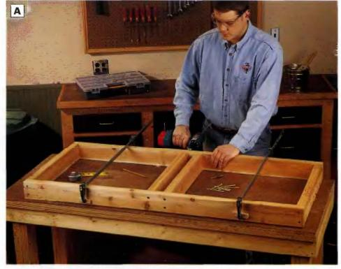
PHOTO A: Bulld the bench seat frame by fastening the front, back, ends and two stretchers together with 3-In. countersunk deck screws.
