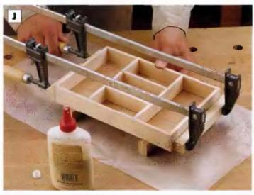
PHOTO J: After the tray dividers are assembled, glue up the tray sides and ends and tack the tray bottom in place with brads.
