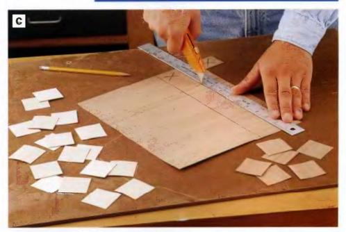
PHOTO C: Lay out and cut the chessboard squares from walnut and maple self-stick veneer. Make 32 of each, using a straightedge and utility knife to cut them out. Hold the blade vertlcally as you cut so that the edges will be square and flt tightly together.
