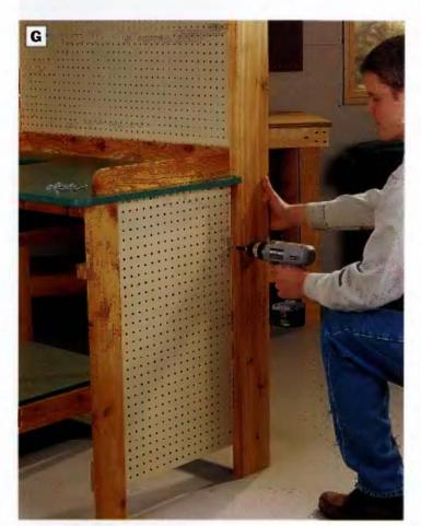
PHOTO G: Fasten the perfboard side and back panels to the bench framework with  $1^{1/2}$ -in. galvanized deck screws. Be careful not to overdrive the screws when installing the perfboard.
