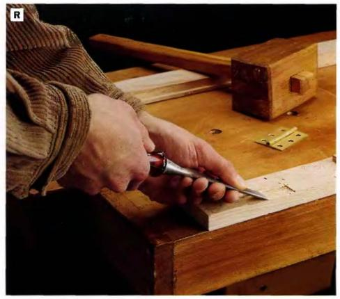
PHOTO R: Chisel mortises for the hinges into the Inside faces of the outer door stiles and Into the front edges of the cabinet sldes. Use one of the leaves from the 21/2-In. butt hinges as a template for tracing the cutting lines for the mortises.
