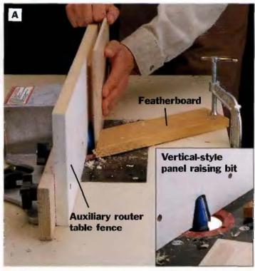
PHOTO A: Rout the raised-panel face of the IId, taking off only about \% In. at a time. Do this by starting with the router fence nearly fiush to the edge of the bit, and move the fence further into the bit for each pass. Removing too much material in one pass could burn the IId panel or prematurely dull the router bit.
