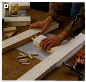
PHOTO D: Use fluted,  $\frac{1}{2} \times 2$ -In. dowel plns to reinforce the joints between the legs and the cross braces.
