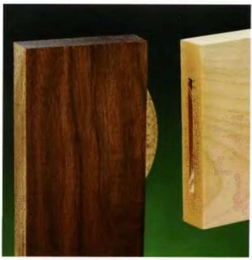
A BISCUIT JOINT is a reinforced butt joint used mostly in casework projects. Made with the use of a biscuit joiner (also called a plate joiner) biscuit joints are quick and easy to make. In addition to reinforcing butt joints in face frames, they are frequently employed to help align and reinforce joints when edge-gluing panels from narrower stock or butting sheet goods together to form a carcase.
