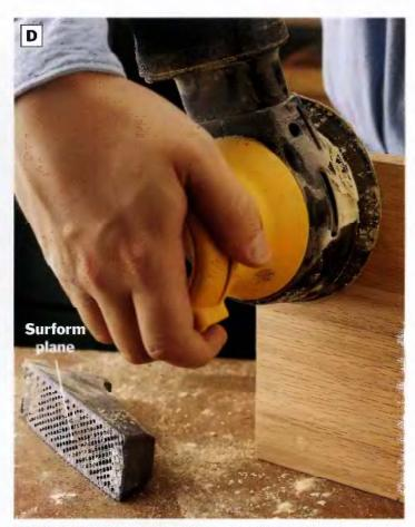
PHOTO D: Shave the piugs so they're nearly flush with the surrounding wood surface using a Surform piane or a wood rasp. Sand away the remaining waste with coarse sandpaper.
