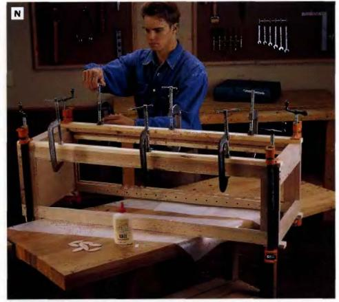
PHOTO N: Attach the face frame to the cablnet assembly with glue and biscuits, and clamp it up with a combination of C-clamps and pipe or bar clamps. Use full-length clamping cauls above and below the cabinet to distribute the clamping pressure evenly over the whole joint and to protect the cabinet parts from damage.
