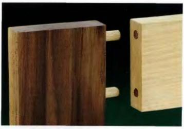
A HIDDEN DOWEL JOINT can be used to reinforce butt joints when assembling face frames or making furniture. The dowels strengthen the joint, and help you align the parts. For best results, use a dowel jig or dowel points for guidance when drilling the dowel holes.
