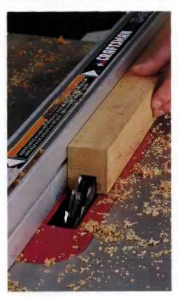
Set the cutting **L**height to the desired dado depth, then adjust the fence so the blade set will start cutting at the shoulder of the planned dado. Make a test cut first, feeding the stock through the blade slowly, with plenty of downward pressure. Use a pushblock when you near the blade. Measure the dado on the scrap and adjust your setup as needed. In harder stock, It's a good ldea to make the cut in multiple passes of Increasing cutting depth.
