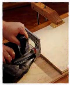
Lay out the position of the two mating parts using a square (note whether you're marking the top or bottom of the workpiece). Set the mating workpiece in position against the mark. Draw a perpendicular reference line on both workpieces at each biscuit location. With the workpieces clamped together and secured to your worksurface, align biscuit joiner with the reference lines and cut the slots in one workpiece.
