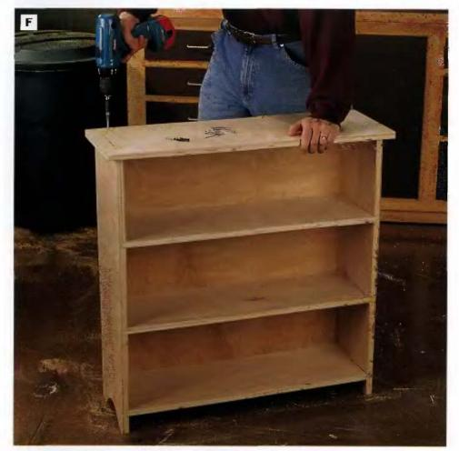
PHOTO F: Position the top panel on the bookcase and fasten it with 2-in. drywall screws driven into countersunk pllot holes.
