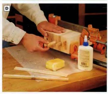
PHOTO D: After your clamps have squeezed the excess glue from the assembly, but before the glue starts to set, remove the waxcoated filler strips In the knlfe slots. Once the glue dries, sand the block smooth.
