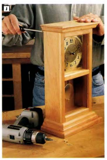
PHOTO J: Apply your finish of choice to all of the wood clock surfaces, then install the clock back with brass fiathead wood screws, driven through the back and into the rabbets in the carcase back.
