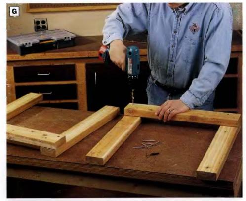
PHOTO G: Make the leg assemblles by fastening each arm support to a pair of legs. Drive pairs of 2½-in. countersunk deck screws through the arm supports and into each leg.
