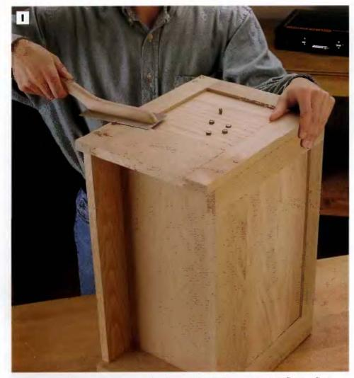
PHOTO I: Use a flush-cutting saw or a dovetall saw to trim the wainut plugs flush. A flush-cutting saw has teeth without set so they won't damage the surrounding wood.
