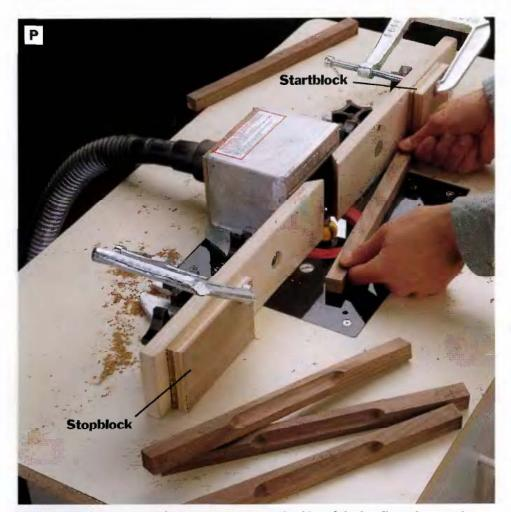
PHOTO P: Rout cove-shaped finger pulis into the undersides of the handles using a router table fitted with a ¾-in. core box bit. Clamp a start block and a stopblock to the table fence to guide your cuts.
