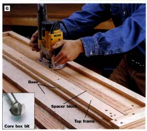
PHOTO G: Rout three flutes into the face frame stilles using a 3%-in. core box bit (See inset photo) in a plunge router. Guide the router against a shop-made jig, which consists of two parts: a base that holds a stille captive and a top frame that serves as an edge guide for the router and establishes the proper position of the two outside flutes. A spacer block attached to the top frame offsets the router to cut the center flute.
