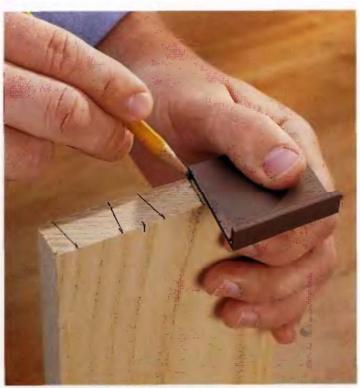
OPTION: Use a flanged dovetall layout jlg to mark the dovetail pins. These Inexpensive little devices can be found in most woodworking stores and catalogs. They're easy to use and yield consistent results. The only real drawback to these jigs is that they're not adjustable, and dovetails aren't a one-size-fits-all joint.
