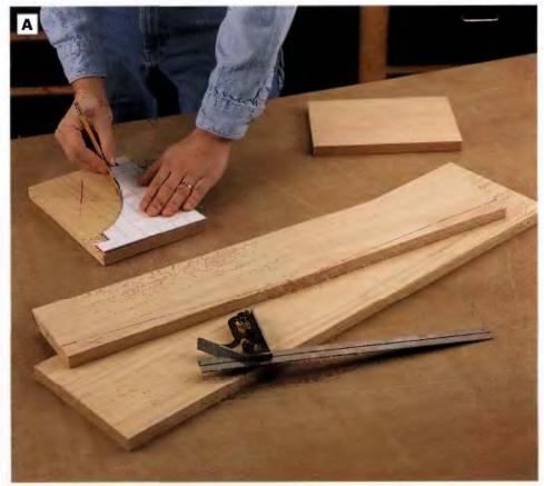
PHOTO A: Lay out the tapered profile on the back panel with a straightedge, and use a fullsize paper or cardboard tempiate as a guide for drawing the curved end profiles.
