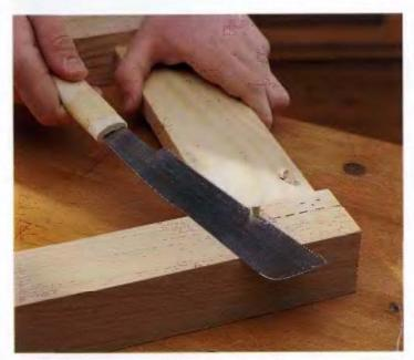
Trim the doweis fiush with the leg surface—here we use a flexible, fine-tooth Japanese-style saw. Depending upon the amount of dowei you need to remove, you may be able to smooth the ends flush with a file instead of sawing them off.
