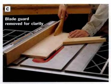
PHOTO C: Cut a 15° bevel into the top edges of the two resawn box boards. Use a featherboard and pushstick for accuracy and safety.
