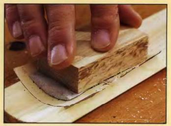
Remove the moided auto body filier and hot-glue a block of wood to the flat face to give the sanding block greater rigidity and durability. Wrap a piece of sandpaper around the shaped face and start sanding. Note: This technique also works with convex sanding profiles.
