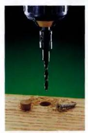
A COUNTERBORE BIT can drili a pilot hole, shank hole and counterbore hole all at the same time.
