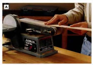
PHOTO A: The side pieces of both the lid and the box get tapered on one end to minimize the thickness of the overlap after they are bent to shape. Begin the taper about 2 in. in from one end of each part. A stationary belt sander works well for sanding these tapers.
