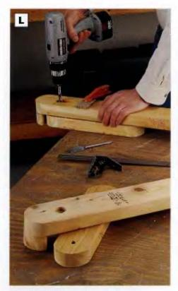
PHOTO L: Drill holes through the foot rest ralls and the legs. The parts will attach with bolts so the legs can pivot on the ralls.
