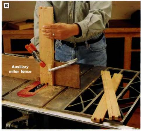
PHOTO B: Mill the finger joints with a ½-in.-wide dado blade. Attach an auxiliary wood fence to the miter gauge to hold the workpieces securely. Since the fingers match on like workpieces, clamp them in pairs to cut the fingers in both parts at once. Note: Work carefully when setting up these cuts—even slightly misaligned cuts can produce poorly fitting finger joints.
