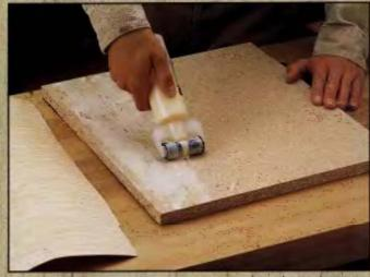
A GLUE ROLLER is used to apply an extremely even coating of glue en large, broad surfaces, such as when applying veneer.
