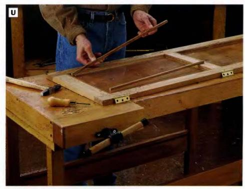
PHOTO U: Set the glass panels in place in the doors and secure them with  $\frac{1}{4} \times \frac{3}{6}$ -in. oak retainer strips. Use 1-in. whre brads driven into pllot holes to fasten the strips to the inside edges of the rabbet grooves in the door frames.
