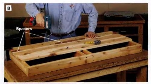
PHOTO B: Install the seat slats on the bench seat frame with screws. Position the back seat slat 7 in. from the back of the seat frame. Insert ¼-in. temporary spacers between the slats before screwing the slats in place.
