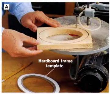
PHOTO A: Draw the frame shape onto 34-in. oak stock, then cut out the frame on the scroll saw. We made a hardboard template to trace this shape and to keep on hand for making more frames. Drill a starter hole for the blade in order to cut out the center of the frame.
