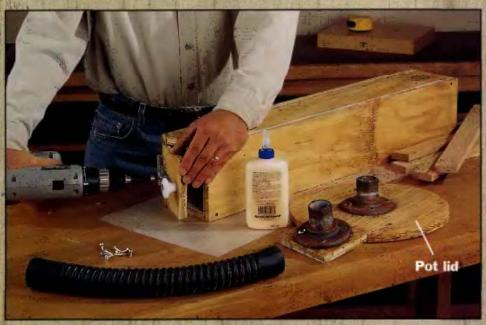
Construct the steamer jig from exterior-grade plywood, moisture-resistant wood glue and galvanized deck screws. Install a hinged door on one end of the steamer box, and drill a 2-in.dla. hole in the other box end and the plywood pot lid for installing a length of heat-resistant or automotive radiator hose. Attach the hose to the steamer box and put lid. We used metal fittings and threaded plpe for making these hose connections.
