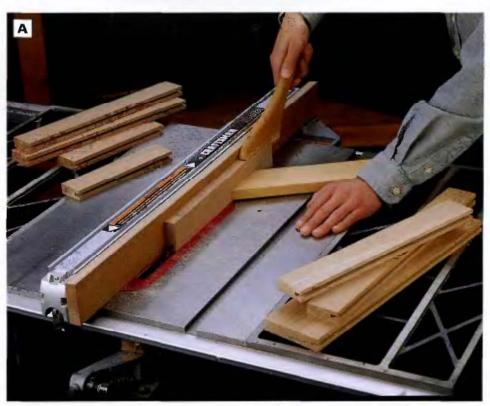
PHOTO A: Cut  $1/4 \times 1/2$ -in. grooves in the edges of the side and back rails and stiles. The grooves should be sized so the plywood panels fit into them snugly. Using a featherboard and pushstick, cut the grooves by making multiple passes with the table saw blade.
