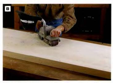
PHOTO B: Flatten the top and bottom surfaces of the benchtop, using a belt sander or a hand plane.
