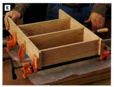
PHOTO E: Spread glue on the mating surfaces of the shelves and sides, and assemble these parts. Note: In this photo, the rail notches in the sides are facing down.
