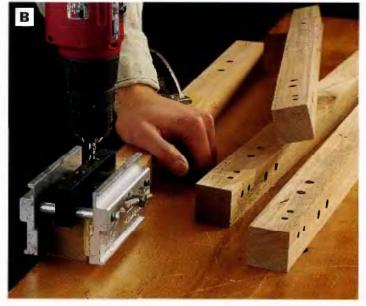
PHOTO B: Drill dowel holes in the legs for the top ralls. Since these joints are not centered on the legs, use a %-in.-thick spacer to offset the doweling jig the proper amount.
