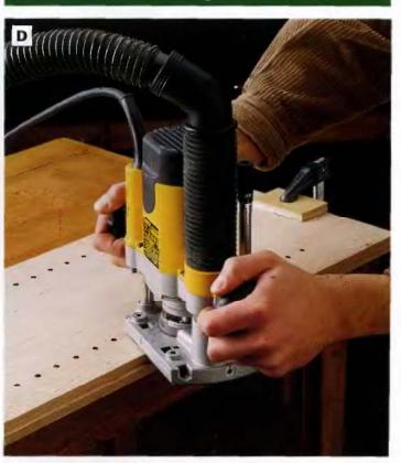
PHOTO D: Cut  $\frac{1}{4} \times \frac{1}{4}$ -in. rabbets Into the back edges of the side, top and bottom panels to create recesses for the back panels. We used a router with a piloted rabbet bit.
