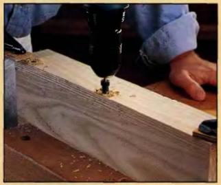
1 Use a counterbore bit to counterbore the pilot hole for the screw (3/8 in. is the standard counterbore diameter).
