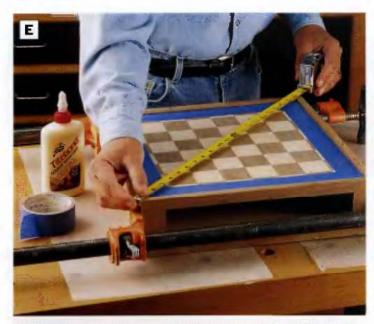
PHOTO E: Assemble the top and bottom, front, back and sides with #0 biscuits and glue to form the carcase. Protect the perimeter of the veneer top from glue squeeze-out with masking tape. Be sure the carcase is square when you clamp by measuring the diagonals. When the diagonal measurements match, the carcase is square. Adjust the clamps, if needed, to adjust for square.
