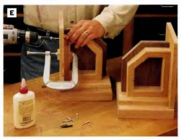
PHOTO E: Position the front plates on top of the bases, clamp them in place and attach them to the frame/divider assemblies with glue and four 1¼-in. flathead wood screws.
