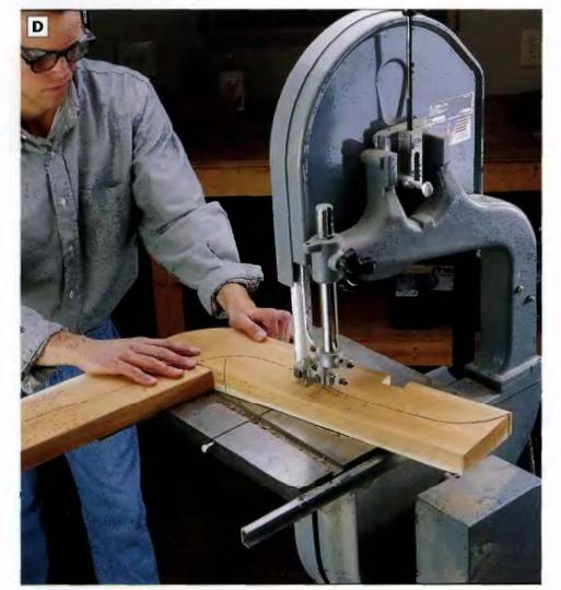
PHOTO D: Use a template to transfer the patterns of the back supports and seat supports onto the glued-up blanks, and cut out the shapes with a band saw or jig saw.
