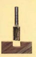
STRAIGHT BIT. Cleans up edges, cuts grooves, can be used for mortising and carving. Most have 2 flutes. Available sizes: 1/4, 5/16, 3/8, 7/16, 1/2, 9/16, 5/8, 3/4, 7/8, 1 in.; 1/2 in. shank only: 13/8, 11/4, 2 in.
