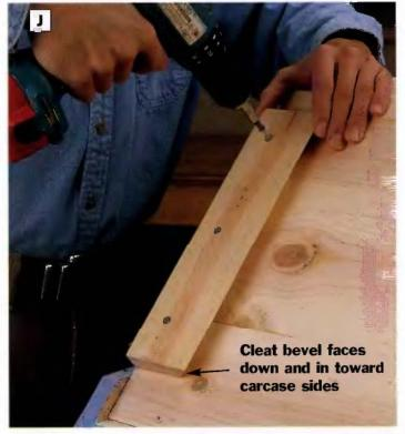
PHOTO J: Attach French cleats to the sides of the cablnet, flush with the top of the carcase. The cleat bevels face down and into the sides.
