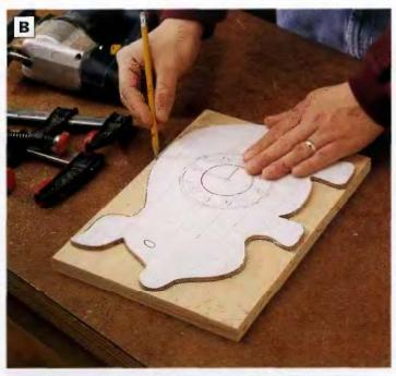
PHOTO B: Trace the template shape onto a plece of plywood, then cut out the clock back with a jig saw.
