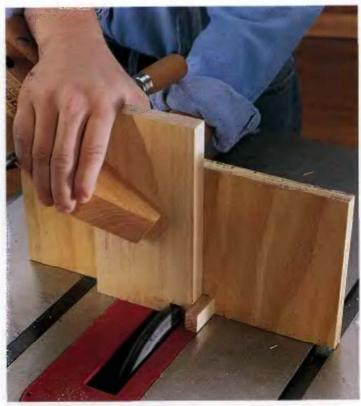
With the pin spacer inserted in the fence siot and the fence in position, butt the first workpiece against the strip and make the first pass. You can hold the workpiece in place by hand or clamp it to make the cut. After the workpiece and fence clear the blade, shut off the saw and back the workpiece off.
