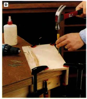
PHOTO D: Giue, ciamp and naii the drawer bottom and back together. Drive the naiis through pilot holes, and recess the naiiheads with a naiiset.
