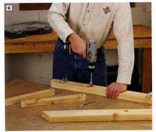
PHOTO G: Bore a 1-in-dia. hole through each back rail for the back rest dowel and a <sup>3</sup>/<sub>8</sub>-in.-deep counterbore for the heads and washers of the adjustment brace pivot bolts.
