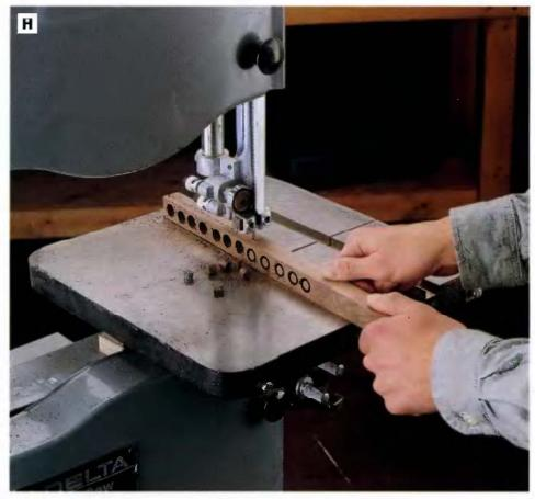
PHOTO H: Cut 16 to 20 piugs with the piug cutter, then resaw the wainut stock to about %in. thick to release the piugs.
