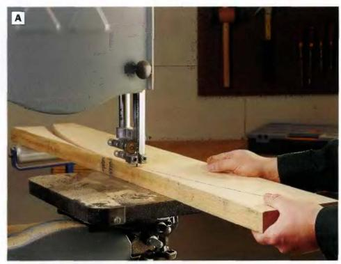
PHOTO A: Cut the profile on the upper back rall to shape on the band saw. Save the curved cutoff pieces to use as cauls when you clamp the back rails and slats together later.
