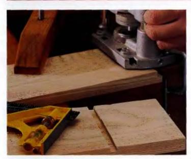
CUT THE DADOES FIRST at the joint locations, using a straight router bit or a table saw and dado-blade set. Measure the dadoes and use the measurements as a guide for cuttling rabbets with lips that fit exactly into the dadoes (in the photo above, a guide block is clamped to the router base and the rabbet cut is made with a straight bit). Make sure the rabbeted ends will not extend more than halfway into the dadoed board.
