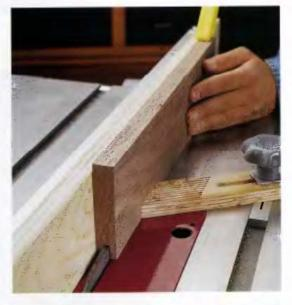
On the Luncut mating board, remove the waste wood on one side of the tongue area. Any rabbetcutting technique may be used with either a standard blade or a dado blade.
