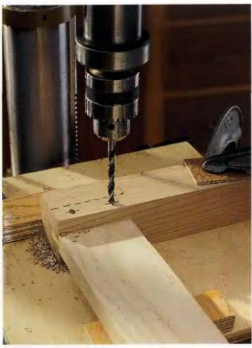
2 Punch a small starter hole at the centerpoint of each pin hole. If your project is a manageable size, use your drill press to drill the holes, as we did in the photo above. Using a brad-point bit will ensure that the hole starts precisely in the centerpoint. Drill the holes all the way through the tenon and into the other side of the mortise. Use a bit stop if your plan calls for stopped pins. If you're creating throughpin joints, drill all the way through the joint and into a piece of scrap.
