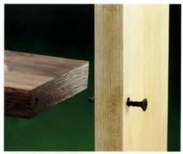
A BUTT JOINT can be used in just about any woodworking situation. If it will undergo stress or pressure, it's a good idea to reinforce the glued butt joint with a fastener, such as a screw.
