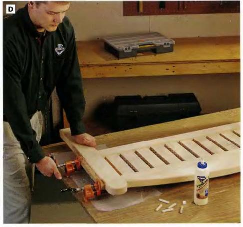
PHOTO D: Complete the back assembly by attaching the stiles to the back rails. Fasten the stiles to the ends of the rails with pairs of doweis and moisture-resistant wood give.
