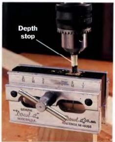
Sllp the doweling Zjlg over each mating edge. Align the mark on the jig corresponding to the dlameter of the dowel hole with each location line you drew on the workplece. Drill a dowel hole the same dlameter as the dowel at each markuse a depth stop to keep the holes of unlform depth (masking tape will suffice if you don't have a depth stop collar).
