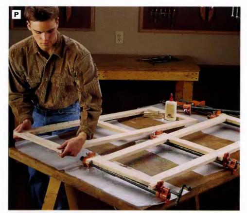
PHOTO P: Make dowel joints at all the rail/stile joints on each cabinet door, then glue the joints and assemble the door frames. Position a bar or pipe ciamp beneath each rall location and use clamp pads to protect the wood.
