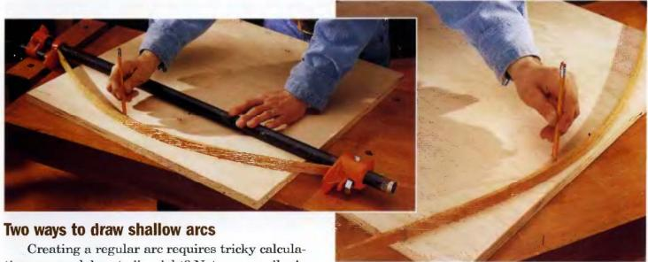
Creating a regular arc requires tricky calculations or an elaborate jig, right? Not necessarily. A trio of nails and a strip of wood will do the job. Tack one nail at each endpoint of the arc, and tack the third nail at the apex of the arc, spaced evenly between the endpoints. Cut a thin strip of plywood or hardboard that's at least a few inches longer than the length of the arc. Bend the strip between the nails as shown in the above, right photo. Trace
