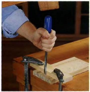
Score along the scribed baseline with a chisel to prevent tearout when you remove the waste around the pins. To ensure a straight scored line, clamp a block of wood next to the scribed line and use it as a chisel guide.
