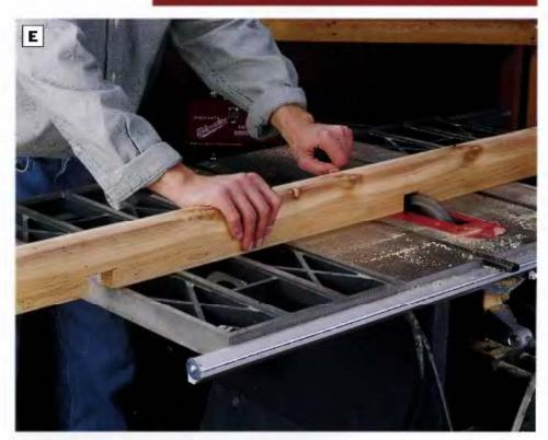
PHOTO E: Cut 11/2-in.-wide notches on the top edge of the cross support. The notches fit together with the notches cut into the bottoms of the seat supports.
