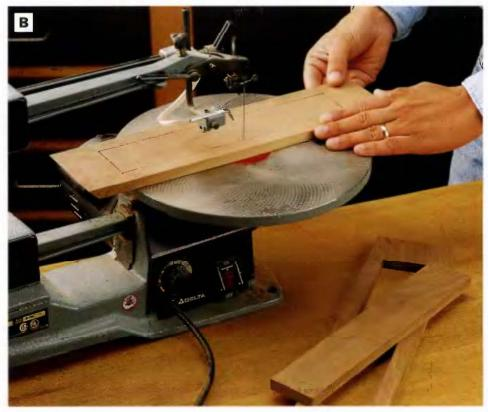
PHOTO B: After drilling starter holes at all four corners of both drawer faces, carefully cut out the faces from the front and back workpleces. The faces are cut from the front and back parts so the wood grain will match when the drawers are closed.
