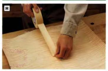
PHOTO H: Tape the jointed edges of the veneer together. Use short strips of tape to hold the joint tight. Then lay a strip down the entire length of the seam.
