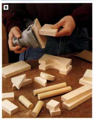
PHOTO B: Sand the blocks thoroughly to remove all sharp corners, edges and any splinters.
