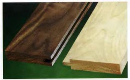
TONGUE-AND-GROOVE JOINTS are fashloned by cutting a centered tongue in the edge or end of one board that fits into a centered dado or groove on the mating workplece. By centering the tongue and fitting it into a centered dado or groove, the shoulders on the tongue side of the joint completely hide the slot made by the dado or groove—a real advantage for concealing the slot-slde of the joint.
