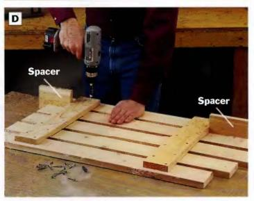
PHOTO D: Arrange the back slats facedown on the bench, and fasten the back stretchers to the slats with 1<sup>1</sup>/<sub>4</sub>-in. galvanized deck screws. Insert <sup>3</sup>/<sub>4</sub>-in. scrap spacers between the slats to make alignment easy.
