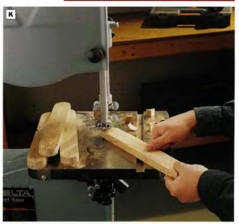
PHOTO K: Cut the four glider arms to shape on the band saw. Both ends of the arms receive 7/8-in.-radius curves. Sand the cut edges smooth and round them over with a router if you wish.
