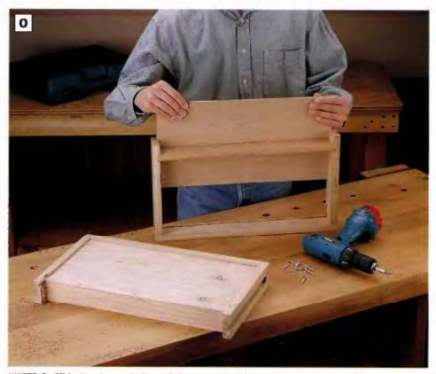
PHOTO 0: Slide the drawer bottoms into the grooves in the drawer sides and front. Secure the drawer bottoms with three screws driven through the drawer bottom and into the bottom edge of the drawer back. Do not use glue.
