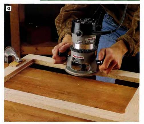
PHOTO Q: Rout a  $44 \times 36$ -in.-deep rabbet recess around the perlmeter of each opening in the upper cablnet doors, Use a ¼-in, piloted rabbet blt (See page 137) to make the cuts, Square off the rounded corners left by the router blt, using a sharp chisel. To keep the wood from tearing, score along the chisei lines with a sharp knife before squaring the corners.
