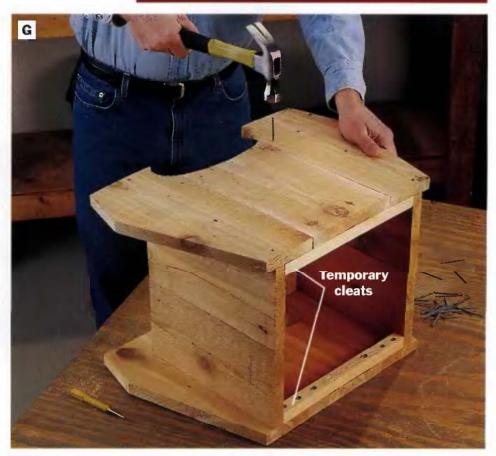
PHOTO G: Fasten the sides to the end/bottom assembly by nailing through the sides and into the ends and bottom. Drill pllot holes before you drive the nails to keep the cedar from splitting. Once both sides are attached, remove the temporary cleats.
