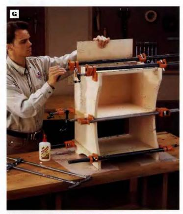
PHOTO G: After gluing and clamping the carcase together, slide the back into the side panel and bottom grooves. Loosen the clamps a bit and adjust the carcase as necessary to square it up so the top edge of the back is flush with the top edge of the rear top stretcher. Then re-tighten the clamps and nail the back to the rear top support with three or four 1-in. brads. No glue should be used with the back panel.
