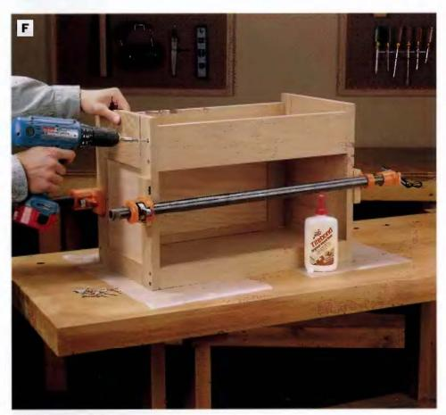
PHOTO F: Giue up the frame-and-panel assemblies and the chest bottoms to create the chest carcase. Reinforce the joints by driving screws through the side panels and into the ends of the front and back rails. Counterbore the pilot holes to accept %-in.-dia. wood piugs.
