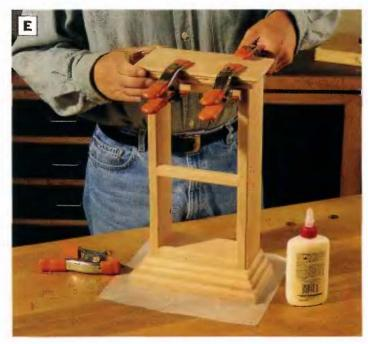
PHOTO E: Glue up the crown and base first, then glue these completed assemblles to the clock carcase. Glue alone will bond these parts sufficiently, so no additional fasteners are needed.
