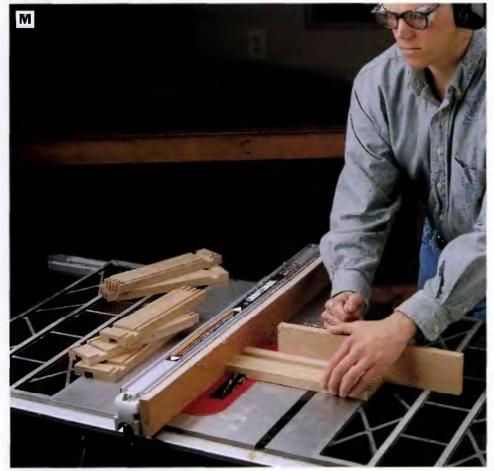
PHOTO M: Cut the drawer back dadoes on the table saw with a dado biade, miter gauge, and rip fence. Push the stock across the biades carefully to avoid binding the workpiece between the blades and the rip fence. Remove the stock after it has cleared the biades.
