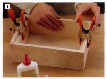
PHOTO I: Glue the tray supports to the inside ends of the box.
