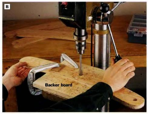
PHOTO B: Bore the <sup>3</sup>/<sub>4</sub>-In.-dia. leg pivot and lock dowel holes in the legs. These holes must be drilled straight through the legs, or the dowels will be difficult to align during assembly. Bore the holes with a drill press, or mount your drill/driver in a right-angle drill guide. Set a backer board beneath each workpiece before you drill, to keep the bit from tearing out the wood as it exits.
