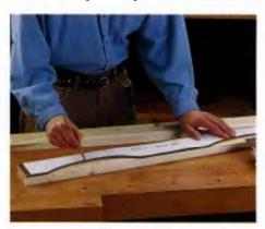
MAKE A STURDY TEMPLATE from hardboard or another durable material when making multiple parts with the same profile.
