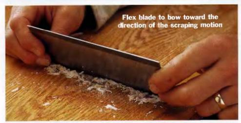
TO USE A CABINET SCRAPER, hold the ends and press in with your thumbs to cause a slight flex. Hold the scraper at a fairly steep angle and push it away from yourself, applying downward pressure as you push (you can also flex the scraper inward and draw it toward yourself).
