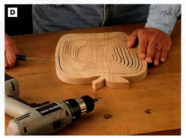
PHOTO D: Fasten the stand and the basket to the frame. Attach the basket with two ¾-in. brass flathead wood screws, driven into countersunk holes in the frame sides. Attach the stand to the frame with a 1-in. brass flathead wood screw, driven up from below.
