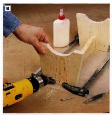
PHOTO B: Giue and ciamp the stretcher between the iegs so the top ends and edges of the parts are fiush. Fasten the parts with countersunk 2-in, flathead wood screws.
