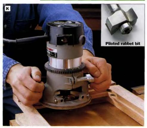
PHOTO K: Use a 3/8-In. piloted rabbet blt (See inset photo) to cut rabbets on the Insides of both side frames and the door frame. The rabbets create recesses for the glass panels. Make several passes of increasing depth with the router, until you reach the final depth (1/2 in). Then square the rabbet corners with a chisel.
