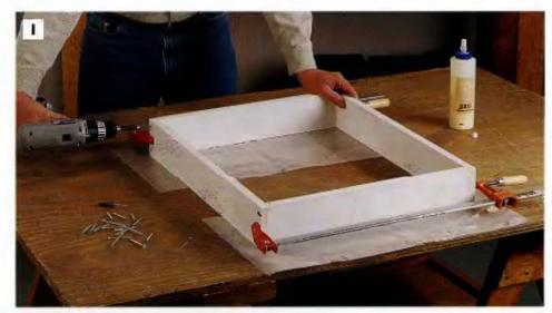
PHOTO I: Glue and screw the drawer ends to the side pleces, driving the screws through countersunk pilot holes to keep the plywood from splitting. Then, fasten the drawer bottom to the bottom edges of this drawer frame. Use the bottom as a guide for squaring up the drawer.
