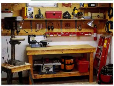
THE BASEMENT SHOP: The basement offers many advantages as a shop location. It's accessible yet set off from the rest of the house, and the essential house systems are right there. Drawbacks tend to be limited headroom, negligible natural light, concrete floors and overall dampness/poor ventilation.
