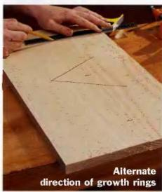
Arrange the jointed boards together to get the most pleasing match of the different grain patterns. This can take some trial and error. Tip: alternate the direction of the growth rings at the ends of the boards. This helps keep the panel from cupping. Once you've got all the boards arranged to your satisfaction, draw a "V" across all joints in the panel. Use the legs of the "V" to maintain your alignment as you glue-up the panel.
