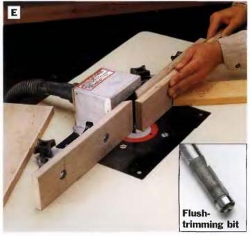
PHOTO E: Trim the 1/8-in.-thick edging flush with the plywood on the shelf, bottom, and front top support using a piloted flush-trimming bit (See inset photo). Secure the workpieces with a featherboard.
