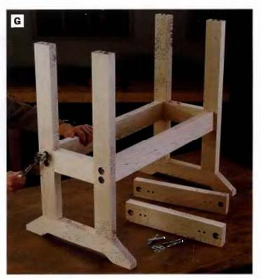
PHOTO G: After pllot holes are drilled, assemble the base with lag screws and washers driven with a socket wrench.
