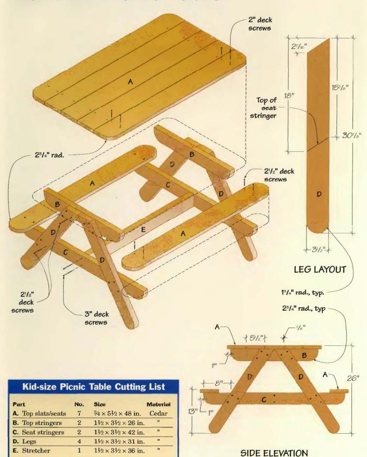
flat to support either the seats or the top slats. Reset your compass to draw a 23/4-in. radius, and scribe the curves on the stringers (See Photo A).
