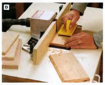
PHOTO D: Rout the roundover and cove and bead profiles into the ends and along one edge of the base and crown parts. Mill the end grain first, then rout the long grain; otherwise the bit could tear out the corners of your finished edges.
