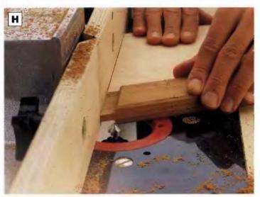
PHOTO H: Rout 1/8-In. chamfers on the ends and edges of the slats using a V-groove bit in the router table. Use an angled pushblock to guide the workplece.
