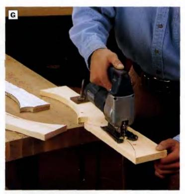
PHOTO G: Make a template of the face-frame rall profile and use it to lay out the curves on the ralls. Cut the profiles using a jig saw, band saw or scroll saw.
