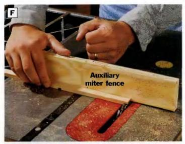
PHOTO F: Cut rabbets and dadoes into the retainer stiles for the retainer rails. Make these cuts on the table saw with a dado blade, and hold the parts against the miter gauge. We installed an auxiliary fence on the miter gauge to keep the dado blade from tearing out the grain on the retainer stiles.
