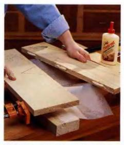
Appiy glue to one edge of each board to be joined, then squeeze giue into the siots. Commercial glue applicators that reach into the slots are available, or you can simply squeeze the glue in with a regular glue bottle and spread the glue with a popsicie stick. Add the biscuits to the slots on one board, if edge-gluing more than one board at a time, apply the glue and insert the biscuits in every board. Now you're ready to clamp the assembly.
