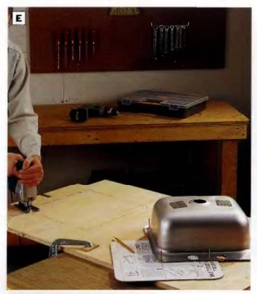
PHOTO E: Center the slnk so it will hang over the storage area on the left side of the bench. Lay out the sink opening using the template provided by the manufacturer, and cut out the slnk opening.
