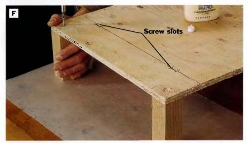
PHOTO F: Attach the foot blocks to the corners of the plywood base with glue and screws.
