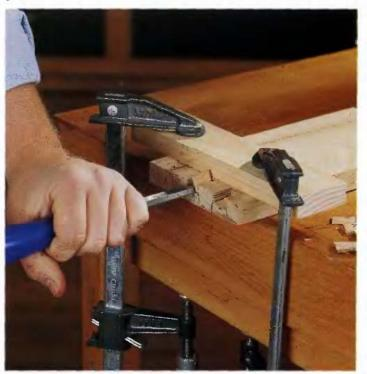
Carefully drive the chisel into the end-grain of the waste area between the pins so the waste wood will break off cleanly at the chisel cut along the baseline.
