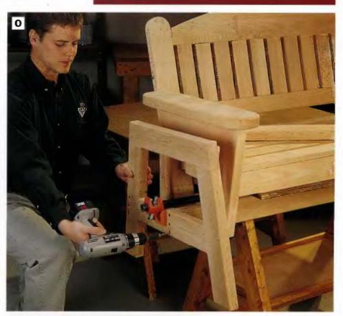
PHOTO 0: Install stretchers between the end assemblies of the glider stand with  $2^{1/2}$ -in. countersunk flathead wood screws. Clamp the stand's ends to hold them stationary as you fasten the stretchers in place.
