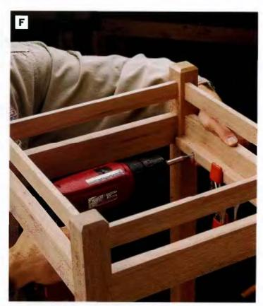
PHOTO F: Attach the tray cleats to the inside faces of the tray ralls, using glue and #6  $\times$  1¼-in. wood screws. The bottoms of the cleats should be flush with the bottom edges of the tray sides and should feature countersunk screw holes for attaching the tray bottom.
