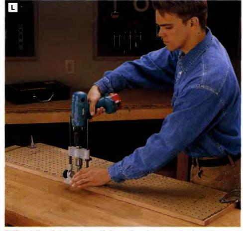
PHOTO L: Drill shelf pin holes in the side frame stiles using a piece of perforated hardboard as a template and a drlll guide to ensure perpendicular holes.
