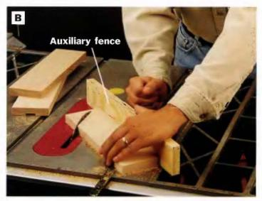
PHOTO B: Mark and trim the angled ends of the strips on the table saw with workpieces supported by the miter gauge set to a 45° angle. Attach a piece of scrap to the miter gauge to serve as an auxiliary fence. Doing so provides better workpiece support and control.
