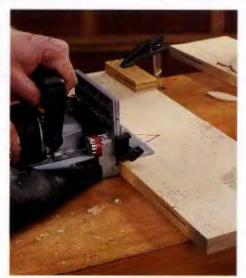
2 Once the boards are iaid out and marked, place them in position and mark the biscuit locations. Use a square to mark all mating edges to ensure that the slots align. Biscuits should be spaced about 8 to 10 in. apart, with a biscuit about 2 in. in from each end. After marking biscuit locations, cut the slots by aligning your marks with the permanent mark on the biscuit joiner.
