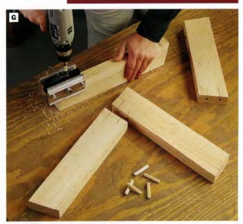
PHOTO G: Join the bench legs to the arm supports with pairs of 2-in. fluted doweis. Use a doweling jig when you drill the holes to be sure that the dowel holes are drilled straight across the joints. Wrap a piece of tape around the drill bit to serve as a temporary depth stop.
