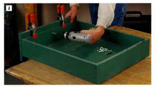
PHOTO J: Clamp the drawer face to the front of the drawer box so the ends of the drawer face are fiush with the drawer sides. The face should overhang the top and bottom of the drawer by  $1^{1}/2$  in. Fasten the drawer face with  $1^{1}/4$ -in. deck screws, driven from inside the drawer.
