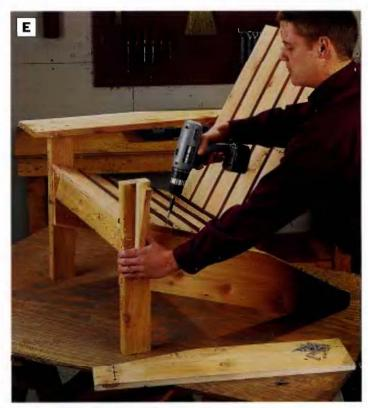
PHOTO E: Set the seat slats in place and insert ½-In.-thlck hardboard spacers between the slats. Remove one chair arm for drlll clearance and fasten the seat slats to the back leg. Once the slats are attached on one side, reinstall the arm, remove the other arm and fasten the slats to the other back leg. Then reinstall the arm.
