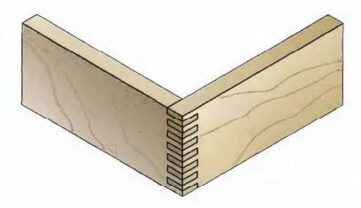
ALSO KNOWN AS BOX JOINTS, finger joints are a good choice for joining two workpieces that are the same thickness. The mating boards in the joint are identical, except that the notches are offset the thickness of one notch on one of the boards. A table saw with a jig can be used for cutting finger joints. You can also use a router (you can buy specialty finger-joint shapers) or a radial arm saw with the biade spinning on a horizontal plane.
