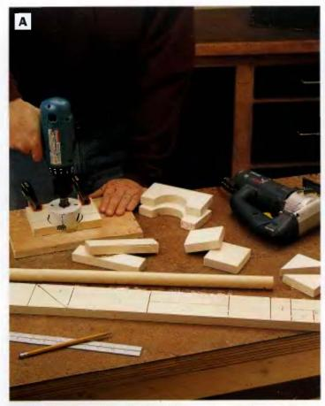
PHOTO A: Lay out and cut the block shapes. Arrange the parts on your boards to maximize the lumber. We cut the curved profiles of the arch blocks with a 3-in. hole saw.
