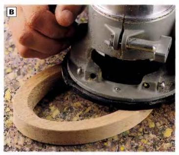
PHOTO B: Mill the 45° chamfer on the Inside edge of the frame with the router held free-hand. Use a non-slip pad beneath the workplece while you rout. Then turn the frame over, switch to a ¼-in. piloted rabbeting bit and rout the back rabbet around the inside edge.
