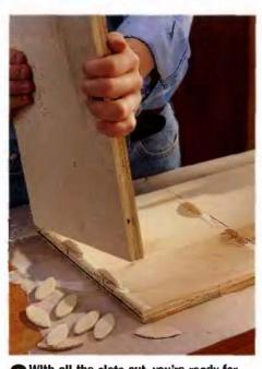
With all the slots cut, you're ready for assembly. Apply glue in the biscuit slots and on the mating surfaces. Insert all the biscuits into the slots in one workpiece, then slip the mating workpiece into position so the parts butt together cleanly. Clamp the parts together, check for square and adjust the clamps as necessary to square up the joints.
