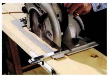
ADJUSTABLE RIPPING FENCE: Most circular saws come with an adjustable ripping fence that attaches to the foot of the saw. The fence rides along the edge of the board to guide the saw so it cuts a line parallel to the board edge. These accessories are fine for rip cuts that don't demand a high level of accuracy.
