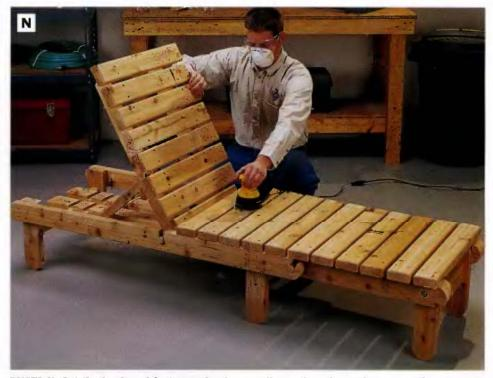
PHOTO N: Set the back and foot rests in place on the seat, and test the action of the parts. Then sand all exposed surfaces of the chair with medium-grit sandpaper. If you sand in an enclosed place, wear a particle mask. Cedar dust can be irritating to your nose and lungs.
