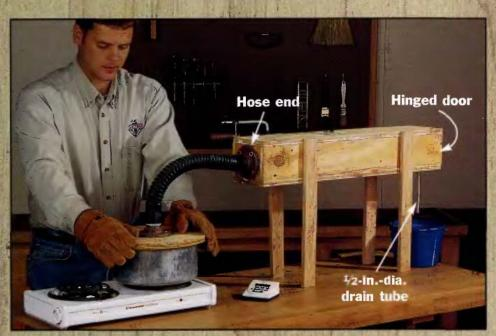
Attach a drain tube through a hole in the bottom of the jig near the door to let excess steam and condensed water vapor escape into a pail. Elevate your steamer on legs until it is higher than the pot to minimize bending the hose. This way, steam can rise and pass more easily into the box.
