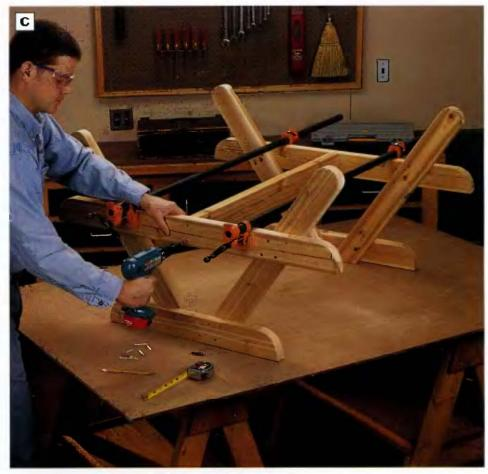
PHOTO C: Stand the leg assemblles top-down to attach the stretcher between them. Hold the stretcher in place with clamps so It is centered on the length of the seat stringers. Drive countersunk 3-In. screws through the seat stringers and into the ends of the stretcher.
