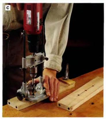
PHOTO C: Drill dowel holes in the bottom shelf rails. We used a portable drill mounted in a portable drill guide equipped with a depth stop. Use a brad-point blt.
