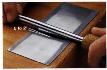
With the scraper lying fiat on a worksurface, rub across the edges of the scraper with a burnishing tool heid at a very slight angle. If you don't have a burnishing tool, any piece of round hardened steel (like the top of a chisel shank) will do. The edge of the scraper should be set back just slightly from the edge of the worksurface to prevent you from burnishing at an angle that's too steep.
