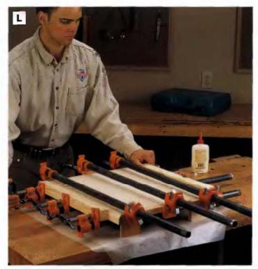
PHOTO L: Giue and ciamp the edging to the tabletop, using #20 biscuits to keep the parts aligned. Match up the miters. Note: The long miters on the wider front edging will protrude past the sides.
