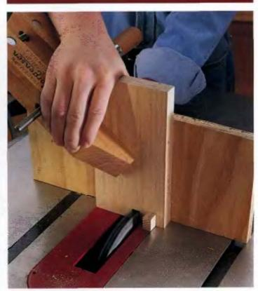
Reposition the workpiece by placing the slot you just cut over the pin space, then make the next cut. Continue in this manner until all the joints in that board are cut. Flip the board end-for-end and cut the fingers on the other end of the board the same way.
