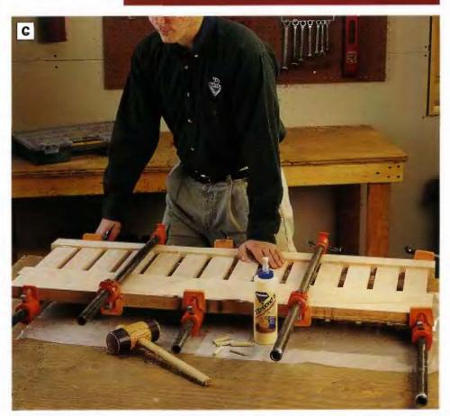
PHOTO C: Assemble the upper and lower back rails and back siats with glue and dowels. Clamp the assembly together, using the waste pieces from Step 1 to make clamping the top rail easier. Alternate the clamps above and below the assembly to distribute clamping pressure evenly.
