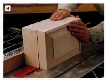
PHOTO H: RIp the box and lid into two pieces on the table saw, with the box bottom against the saw fence. Ralse the blade to 5% in. and cut one end, then cut adjacent sides, working your way around the box.
