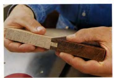
Apply wood glue in the groove, then insert the tongue. The tongue should flt fully in the groove.
