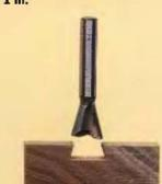
DOVETAIL BIT. Used to cut dovetail joints, generally with a dovetail jig. Angles of flutes vary between 7 and 14°. Available sizes: 1/4, 5/16, 3/8, 1/2, 5/8, 11/16, 3/4 In.; 1/2 in. shank only: 13/16, 1 In.
