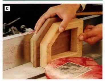
PHOTO C: Flatten the long edges and bottom ends of the frame/divider assemblies on the jointer or sander. The purpose here is to produce flat, even surfaces to attach to the base caps and front plates.
