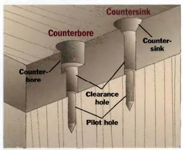
A COUNTERBORE HOLE has a cylindrical top intended to accept a wood screw plug; a countersink hole has a beveled top just deeply enough for the screw head to be driven below the wood surface, creating a small recess to be filled with wood putty.
