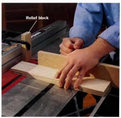
Cut the shoulders of the tongues on a table saw, using the miter gauge to Lefeed each workpiece past the biade. Clamp a relief block to the fence and measure out from its position to the biade to set up the cut.
