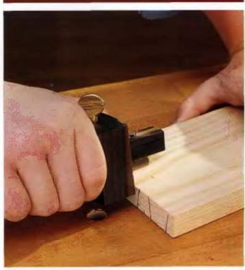
Next, mark the pin length with a marking gauge. This line lets you know how deep to cut, so scribe it well.
