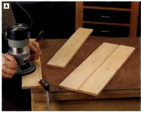
PHOTO A: Rout chamfers along the mating edges of the back slats with a piloted chamfering bit set to a cutting depth of ½ in. It's a good idea to label the slats first so you profile only the edges that will meet once the panel is glued up.
