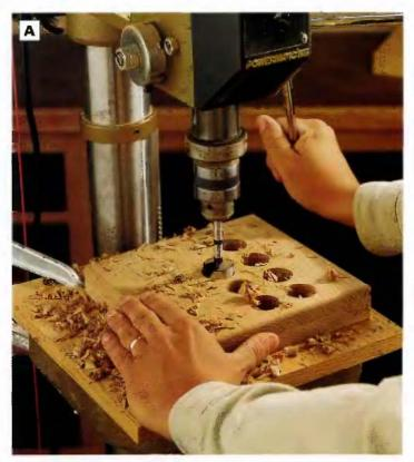
PHOTO A: (Optional) Drill three rows of 1¼-In.-dla. holes into the top face of both bases with a Forstner bit in the drill press. These holes will be filled with ballast and concealed by the base caps.
