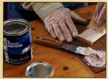
1 Cut a 4- to 6-in. strip of the molding or trim you need to sand. Tack a small piece of scrap wood to each end of the molding strip to create "forms." Fill or cover the molding with auto body filler, smoothing the filler so it's level with the tops of the forms. Let the filler dry according to the manufacturer's recommendations.
