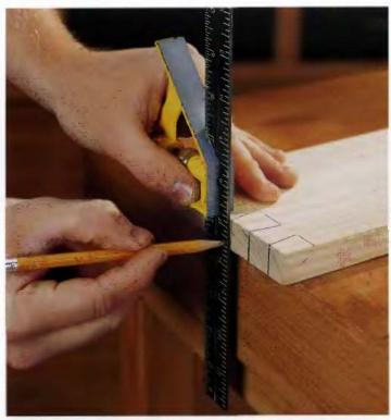
10 Draw straight cutting lines across the end of the tail board, using a combination square or try square. The cutting lines should align with the outline marks transcribed from the pin board.
