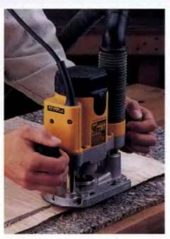
A ROUTER is used to make dadoes and rabbets as well as edge profiles. With special bits and accessories it can also be used for pattern cutting, circle cutting and many other cutting tasks.
