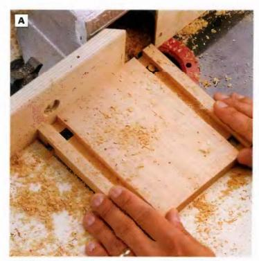
PHOTO A: Make the first series of grooves with the router fence set  $\frac{1}{2}$  in. away from a  $\frac{1}{2}$ -in. straight bit raised to  $\frac{3}{16}$  in. Cut two parallel grooves into one face, then flip the workpiece and cut two grooves in this face that are perpendicular to the grooves in the opposite face. Raise the biade to  $\frac{3}{8}$  in. and then  $\frac{7}{16}$  in., cutting progressively deeper grooves until the intersections between the grooves open up.
