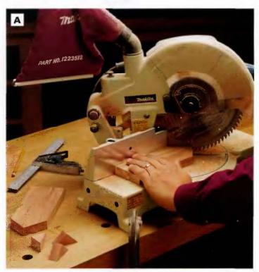
PHOTO A: Trim the gable ends of the sides on a power mlter saw with the blade swiveled to 45°. Center the gable peaks across the width of the workpleces.
