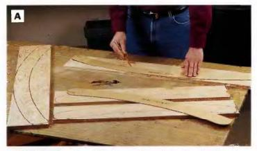
PHOTO A: Create seat and back support templates from hardboard, and use these templates to draw the profiles on the back and seat support workpieces (use treated iumber, not plywood as shown). Cut out the parts with a jig saw.
