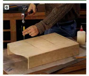
PHOTO G: The back is secured with glue and nalls. Before attaching, mark a line across the back at each shelf to serve as guides for locating the fasteners. Drill pilot holes for the finish nails, and set the heads so they will not scratch the wall once the shelf unit is hung.
