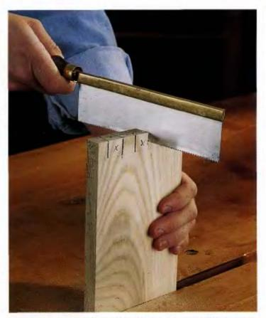
5 Use a tenon saw, also called a dovetall saw, to cut the shoulders of the pins. Split the lines with the saw, favoring the waste side. Cut down to the scribed lines, but do not cut below the lines or the kerf cut will show when the joint is assembled.
