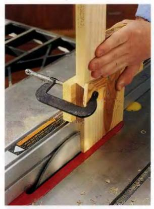
Cut the tongue portion of the iap joint on your table 2 saw, using a tenoning jig to support and guide the workpiece. Set up the saw as if you're cutting a deep rabbet, and begin by making the cheek cuts.
