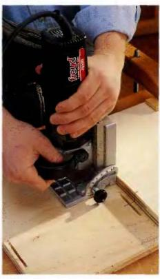
With the workpieces still clamped together, cut matching slots in the other workpiece, using the reference lines to align the biscuit joiner.
