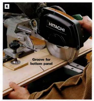
PHOTO K: The sides, front and back for each drawer can be cut from a single 8-ft.-long strip of ½-in. piywood. By cutting the groove for the drawer bottom before cross-cutting the parts, you can ensure that the groove will line up on all four parts.
