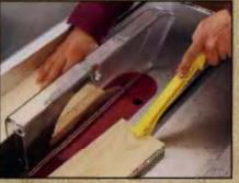
When the biade cuts the board in two, push the workpiece past the biade with your right hand until it clears the blade on the outfeed side. Slide the cutoff piece away from the blade with your left hand or a pushstick to prevent it from coming in contact with the blade.
