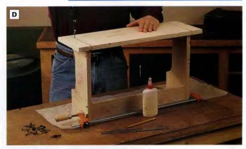
PHOTO D: After the bench stretcher is secured between the legs, fasten the bench seat with giue and countersunk 2-in. drywaii screws.
