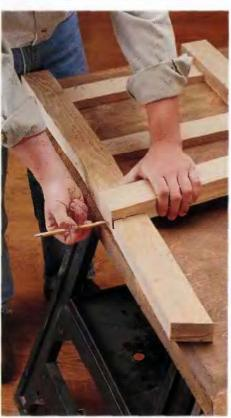
CHAIRS AND BENCHES. Lap joints are very often used to join the arms and/or spreaders of a chair base to the legs. The fitted nature of the joint provides good resistance to downward stress.
