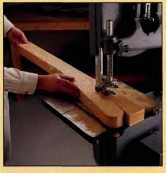
**RIP-CUTTING WITH A** BAND SAW: Like jig saws, a band saw can make "rip" cuts that generally follow the grain of the wood but aren't necessarily straight or paraiiei to the edge of the board. You can also make "true" rip cuts that are parallel to the edge using the fence that comes with most bandsaws. The edges of the cut won't be as sharp as a table saw cut, however.
