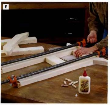
PHOTO E: Use plpe clamps to draw the feet tightly against the bottoms of the legs.
