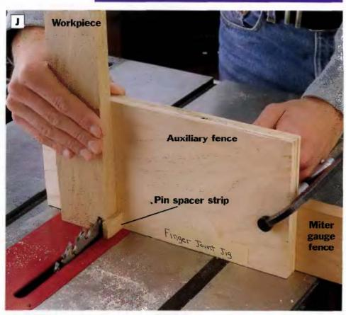
PHOTO J: The jig we used consists of an auxiliary fence clamped to the miter gauge fence. A  $\frac{1}{4}$ -in.-wide  $\times$   $\frac{3}{4}$ -in.-deep slot in the auxiliary fence is filled with a pin spacer strip to use as a gauge for aligning the finger joint cuts. Make the first finger joint cut with the workpiece butted against the pin spacer strip.
