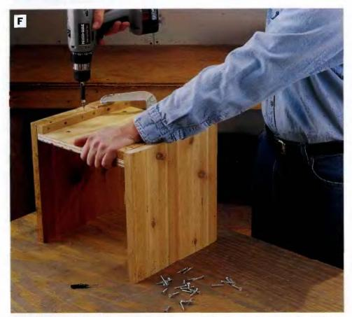
PHOTO F: Cut the bottom plece to size, drill five weep holes through the bottom for drainage, and fasten it to the cleats on the end pieces with countersunk screws. Attach the bottom so it will rest on the cleats when the planter is finished.
