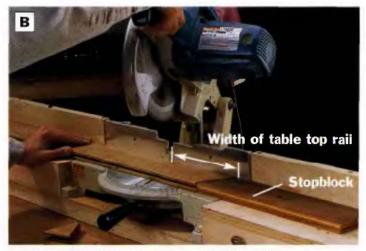
PHOTO B: Cut the tabletop rails to length with a 22½° angle on each end. Attach an angled stop block to the saw table for consistent cuts.
