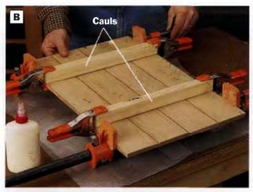
PHOTO B: Glue and clamp the slats together to form the back panel. Clamp scrap cauls across the slats to hold the panels flat. Apply just enough clamping pressure to close the joints.
