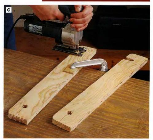
PHOTO C: Connect the lock dowel hole with straight lines to the edge of each stretcher, forming the lock dowel slots. Clamp the legs to your worksurface and cut along these lines. The width of the slots should be 13/16 in., to provide a loose flt for the 3/4-in.-dia, lock dowel.
