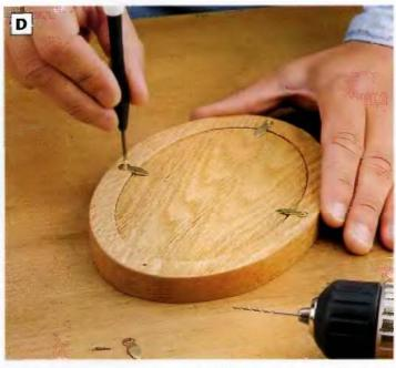
PHOTO D: Four brass turn buttons hold the glass, photo and back in the frame, install the hardware so the turn buttons are spaced evenly around the frame. Drill pilot holes for the tiny turn button screws.
