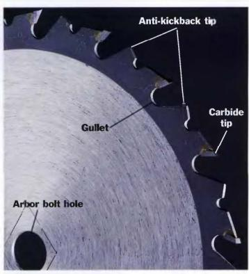
CIRCULAR SAW BLADES are fitted onto portable circular saws, table saws, radial-arm saws and power miter saws. Select blades by matching the number of teeth per inch to the task at hand—but make sure the tpi number is for the correct blade diameter (anywhere from  $3\frac{1}{2}$  in. to 18 in. or so, with  $7\frac{1}{4}$  in. the most common for portable circular saws, and 10 in. the most common for table saws, power miter saws and radial-arm saws).
