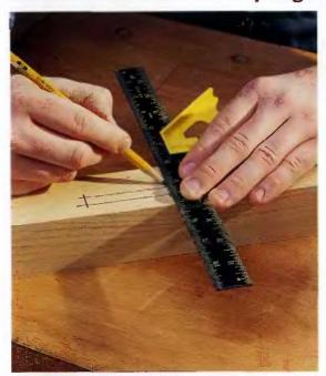
Lay out an outline for the mortise on the workpiece using a pencil and combination square. If you need to make mulitple mortises the same width and in alignment, use a marking gauge.
