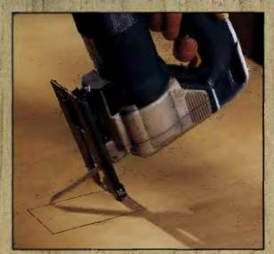
USE A JIG SAW: Tip the Jig saw forward on the front edge of its foot. Align the tip of the blade with the cutting line, then turn on the saw and gently but firmly iower the blade into the cutting area. The blade will want to bounce, but by maintaining firm pressure on the front of the foot you can keep it under control until it enters the wood.
