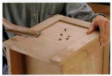
SCREW HOLE COUNTERBORES can be plugged with matching wood plugs or with contrasting plugs that give the project decorative flair, as above.
