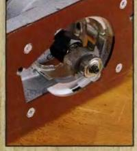
Piloted router bits have a bearing or a fixed spindle that follows the edge of a board as you cut, allowing the cutters to engage the wood and maintain a uniform depth of cut without the need for a straightedge guide. Piloted rabbet bits, like the one shown above, are generally available in sizes that will cut rabbets ranging from ½ in. to ¾ in. deep.
