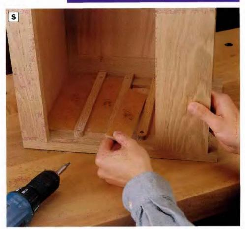
PHOTO S: Mount the drawer sildes using spacers to maintain even placement. After the sildes are in place, remove the spacers.
