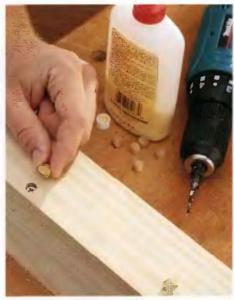
2 After the screw is driven, apply wood glue to the end of a screw piug. Set the piug into the counterbore hole with a wood mallet. For contrast, the grain in the piug should be perpendicular to the workpiece grain. For concealment, align the patterns.
