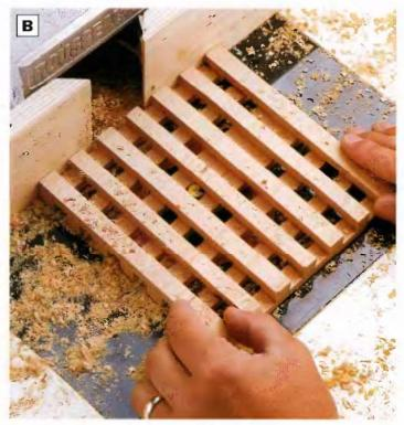
PHOTO B: Reposition the fence at 1½ in. and 2½ in. from the bit for the second and third rounds of cuts. Continue milling the grooves in three passes, raising the bit after each, until the trivet is completed.
