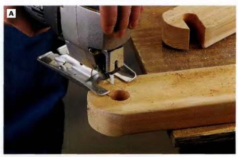
PHOTO A: Cut notches in the seat rails for back rest and foot rest dowels by boring 1-in.-dia. holes in the ralls first, then cutting through the rails to the holes to form the notches. The foot rest notch (shown) is angled 45° on the seat rail, while the back rest notches are perpendicular.
