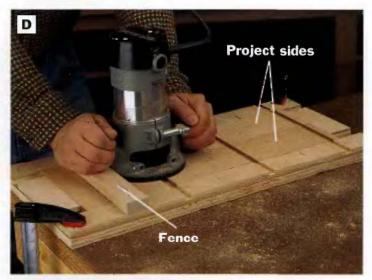
PHOTO D: Create a simple shop-made jlg out of plywood to gang-rout shelf dadoes across the sides. Guide the router base along a removable fence, and rout each dado clear across both the jig and sides.
