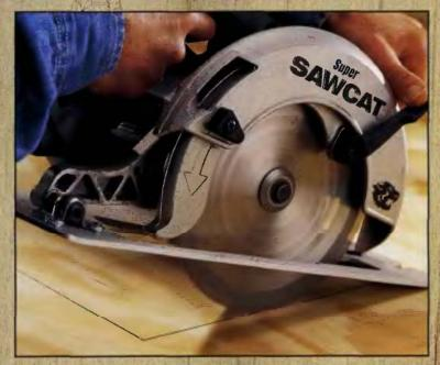
USE A CIRCULAR SAW: Place the front edge of the foot against the board, retract the blade guard and hold it in a raised position with your thumb. Turn on the saw and lower the blade into the wood, using the front of the saw foot as a fuicrum. Aiways wear safety goggles.
