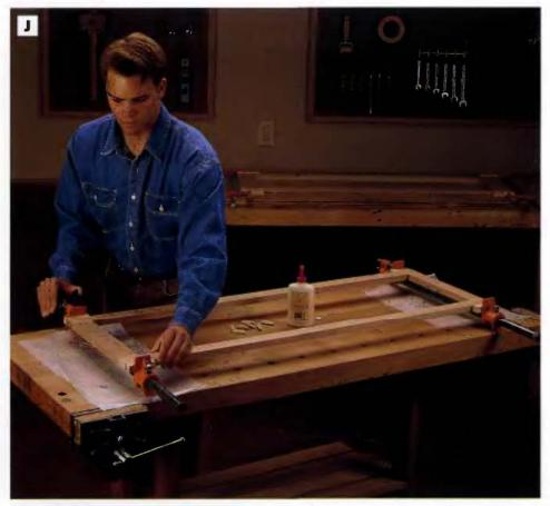
PHOTO J: Glue the dowel joints and clamp together the ralls and stiles for the face frame, side frames and door.
