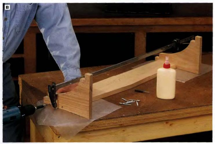
PHOTO B: Fasten the coatrack ends to the back with give and flathead wood screws driven into counterbored pilot holes. Clamp the parts together first to hold them securely while you install the screws.
