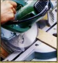
Cut one mating board square, Land cut the other at a 45° bevel, using a miter saw. The beveled board should be slightly longer than the finished length.
