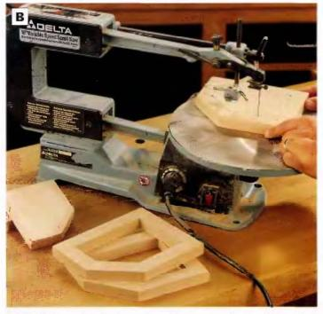
PHOTO B: Lay out and cut one frame to shape on the scroll saw, then use this first frame piece as a pattern for tracing the shapes of the other seven frames. To remove the center cutout from each frame, drill relief holes at each corner of the cutout so you can turn the workplece on the scroll saw as you cut.
