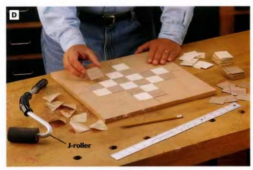
PHOTO D: Divide the MDF top panel Into four layout quadrants with a straightedge and pencil. Then begin to install the veneer squares, starting with a group of four at the center. Work outward from the center, in all four directions, fitting the squares as tightly together as you can. Use a J-roller or rolling pin to press the back of each square firmly in place.
