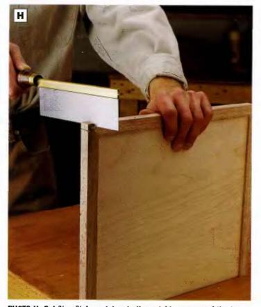
PHOTO H: Cut  $36 \times 36$ -in. notches in the outside corners of the tray to allow it to fit around the inside corners of the legs. Use a small, fine-tooth saw like the dovetall saw shown above. Make sure to keep the tray plumb as you cut.
