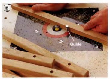
PHOTO B: Ease the edges and ends of the slats and crossbars with a ½-in, roundover bit in the router table. Use a pin-style guide on the router table to help control the workpieces as you machine them.
