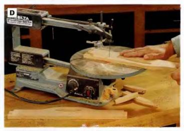
PHOTO D: Cut the curved handle profiles and cutouts on the scroll saw. You'll need to drill an access hole for the blade first, in order to start the handle cutout.
