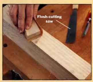
**3** Trim the piug with a chisel, flush-cut saw or rasp, then sand the piug until it's even with the wood surface.
