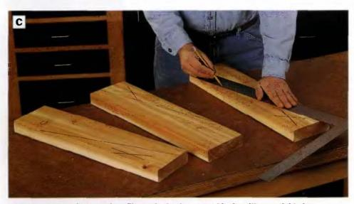
PHOTO C: Lay out the angled profile on the back support blanks with a straightedge.
