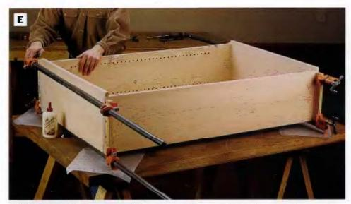
PHOTO E: Assemble the carcases for the upper and lower cabinets. Use pairs of bar or pipe clamps and wood cauls to draw the panels together. Positioning the back panel in the back panel recess serves as a heipful reference for squaring the carcase.
