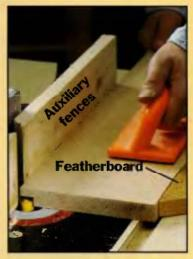
workplece through the bit with a push block or hold-down.
