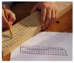
TRANSFER GRID DRAWINGS to your workpiece by drawing a scaled grid, then re-creating the pattern using the grid as a reference.
