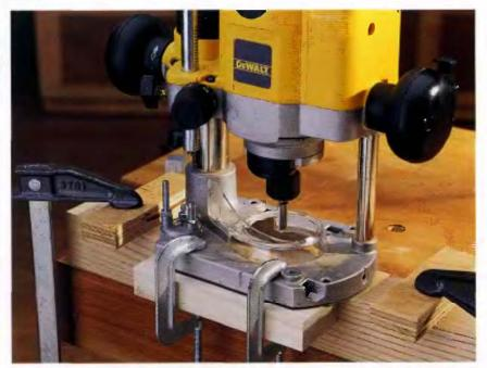
In your plunge router, install a straight bit with a diameter equal to the width of the mortise. Clamp a stop block guide to the router base so the bit aligns with the mortise outline. Set the cutting depth to the depth of the mortise. With the workpiece secured, plunge the bit into the wood and make the mortise cut.
