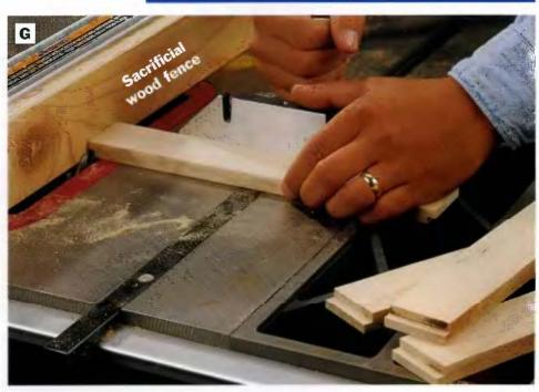
PHOTO G: Attach a sacrificial wood fence to your table saw's rlp fence, and use it to establish the  $\frac{1}{4} \times \frac{1}{4}$ -in. dado blade reveal for cutting rabbets on the ends of the drawer front and back pieces. Cut the rabbets with the workpieces held against both the miter gauge and the sacrificial fence.
