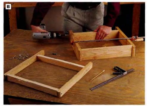
PHOTO B: Build an upper and lower frame for each chair. Note that the end pieces of each frame are inset  $\frac{3}{8}$  in. and  $\frac{31}{8}$  in. from the ends of the side pieces. Clamp the frame parts together, and drive 2-in. galvanized deck screws through the sides and into the ends to make the frames.
