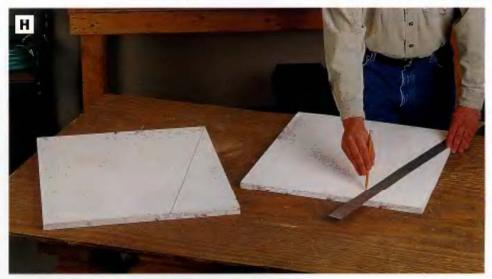
PHOTO H: Cut the cart's angled sides by measuring  $8^{1/2}$  In. along one short edge of each side panel. Connect this point to the top corner on the opposite edge with a straightedge. Cut these parts to shape. Assemble the sides, ends and bottom panel to form the cart box.
