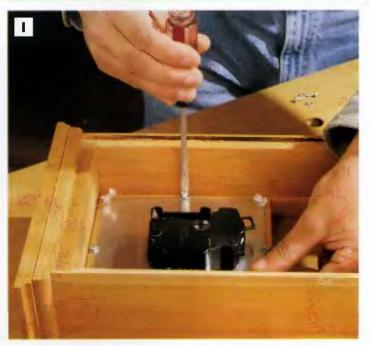
PHOTO I: Fasten the brass clock face to the top portion of the retainer frame with slx panhead sheet metal screws and washers. Pushpins serve as a handy way to hold the clock face in place as you adjust it, prior to installing screws and washers.
