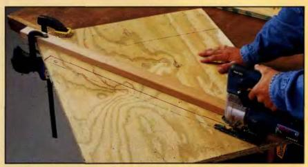
RIP-CUTTING WITH A JIG SAW: One advantage to using a jig saw to make rip cuts is that it's easy to set up a straightedge and make a cut that's not parallel to the edge of the board. Be sure the guide is set to allow for the offset between the saw foot and biade.
