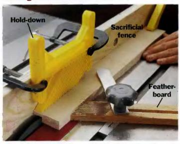
WITH A DADO BLADE SET. A dado blade (See photo, top left) can cut shallow rabbets in a single pass. If the rabbet is deeper than 3/8 in. or the workpiece is hardwood, make the cut in multiple passes. Attach a sacrificial wood fence to the rip fence. Set the fence position and cutting depth, then make the cut. Use a hold-down, featherboard and pushstick to guide the workplece.
