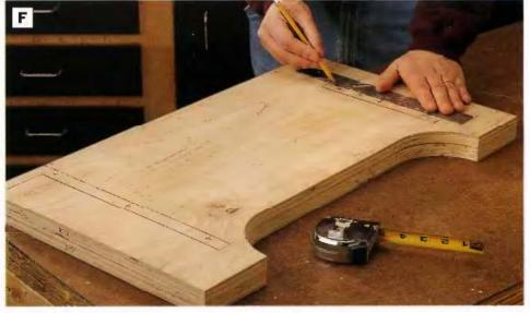
PHOTO F: Lay out the shelf and footrest positions on both sides of both desk legs. See the Side Elevation drawing, page 273, to position these parts.
