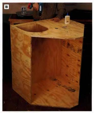
PHOTO B: Fasten the bottom panel in place between the front, back and side pieces with countersunk deck screws. Position the bottom 3 in. up from the bottom edges of the parts and so the top face is flush with the bottom of the door opening.
