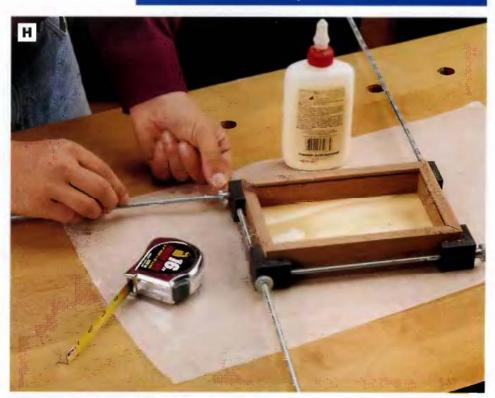
PHOTO H: Giue and ciamp the box parts together, with the box bottom in piace. We used a frame ciamp, which holds all four corners of the box together and squares up the assembly as well. If you use a different ciamping method, adjust the ciamps until the box is square.
