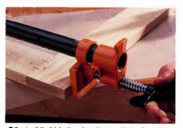
4 Create all the joints, then clamp the assembly together with pipe clamps or bar clamps. Be sure to use a clamp pad between the wood and the clamp jaws so the jaws don't mar the wood. Do not overtighten the clamps.
