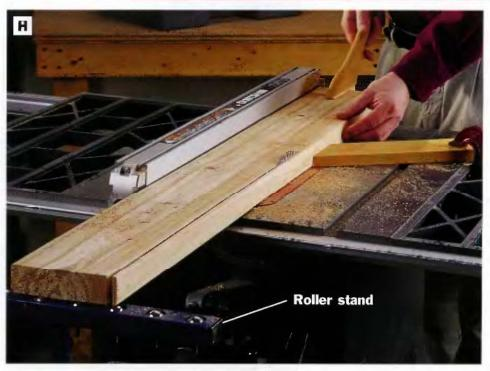
PHOTO H: Rip-cut 2  $\times$  6 stock down to a width of 51/8 ln. to form the tabletop siats. You could make these cuts with a circular saw and straightedge gulde, but a better choice is to use the table saw and rip fence. Support workpleces with a roller stand as they leave the saw table.
