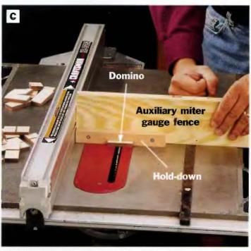
PHOTO C: To trim the domino centeriines, fasten a notched hoiddown to an auxiliary fence mounted on the table saw miter gauge. The hoiddown keeps your hands a safe distance from the biade and aligns each domino accurately to make the shallow centerline cut. Cut a centerline across one face of each domino.
