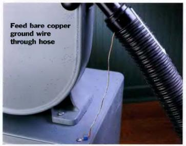
Due to the dangers of sparking caused by static electricity, a dust collection system should be electrically grounded so the built-up electricity can escape. Attach a strand of bare copper wire to the metal cabinet of each stationary tool in the dust collection system (assumes that tools are grounded through the power supply system). Drill a small guide hole into the hose port near the tool and feed the wire into the hole.
