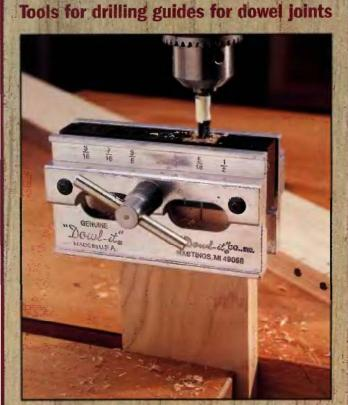
A DOWELING JIG makes drilling accurate dowel holes a breeze. The jig is set to match the thickness of the workpieces, then fitted over each workpiece individually to guide the drill bit and ensure that the dowel holes align when the workpieces are joined. See the step-by-step instructions, previous page.
