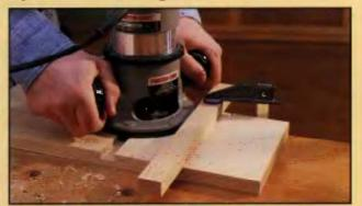
STRAIGHT BIT AND CUTTING GUIDE. A router guide is needed to make a dado or plow with a straight router bit. The simplest guide is a plain, straight board clamped to the workplece the correct distance from the cutting line.
