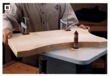
PHOTO B: To smooth the profiles on the sides (and to make them Identical), we clamped the sides together and gang-sanded them on an oscillating spindle sander.
