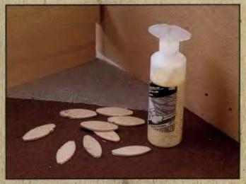
A SPECIAL GLUE TOOL FOR BISCUITS can be slipped into a biscuit siot to deliver glue with no spillage or mess.
