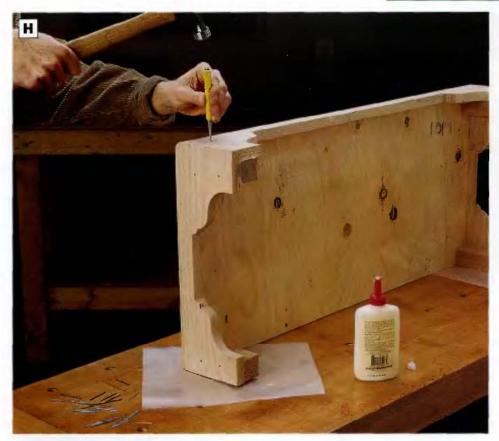
PHOTO H: The trim pieces wrap around the base structure, adding decoration and "feet" to the cabinets. Use 4d finish nails and give to attach the mitered trim pieces. Drill pilot holes for the nails (you can remove the head from a finish nail and chuck it into your drill if you don't have a drill bit small enough for the job). Set nails with a nailset.
