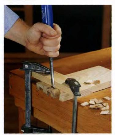
Remove waste in half the area, then flip the board over and continue removing waste from the other side. The beveled face of the chisel should face toward the ends of the dovetails, with the flat face contacting the guide board. When all the waste is removed, clean up the cuts carefully with a smoothing file.
