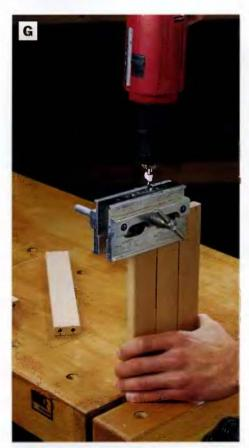
PHOTO G: Use a doweling jig to drill centered dowel holes in the ends of the rails and handle. Clamp ralls together edge-to-edge to provide more surface area for the jig.
