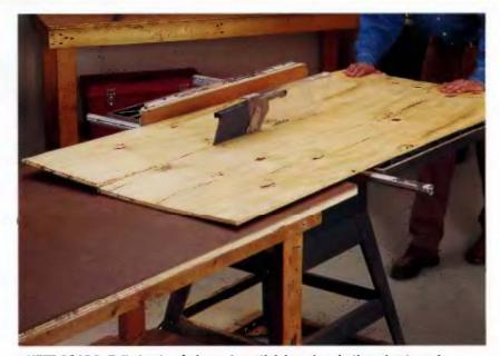
SHEET GOODS: Fuil sheets of plywood, particleboard and other sheet goods can be ripped effectively on a table saw if you position a sturdy table on the outfeed side of the saw, at or just below the saw table surface. But many woodworkers prefer to cut the sheets down to size with a circular saw or panel-cutting saw first.
