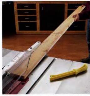
LONG BOARDS: When ripping iong boards, tip the back edge of the board up so it is slightly higher than the saw table. Doing this will press the leading edge of the board firmly down on the saw table. Lower the back edge of the board as the cut progresses.
