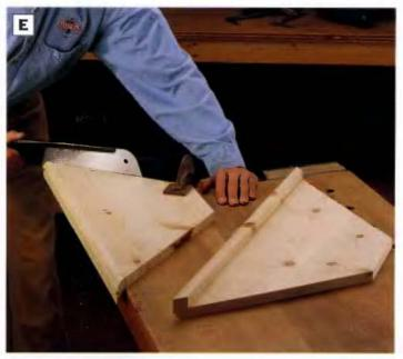
PHOTO E: Clamp the fixed shelves to your workbench and trim the profiled shelf edging to match the angled ends of the shelves. We used a fine-toothed Japanese-style pull saw to make the cuts.
