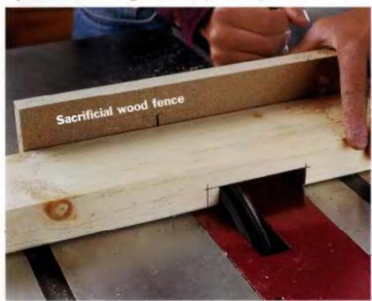
USE A DADO BLADE. A dado biade set installed in your table saw is the fastest tool for cutting notches in stock to create lap joints. Set the dado blade to its maximum cutting width and set the cutting height to equal the depth of the notch. Attach a sacrificial wood fence to the miter gauge for your table saw. Hold or clamp the workpiece securely against the fence so the area to be notched is clear of the miter gauge. Cut through the stock and the fence in severai passes.
