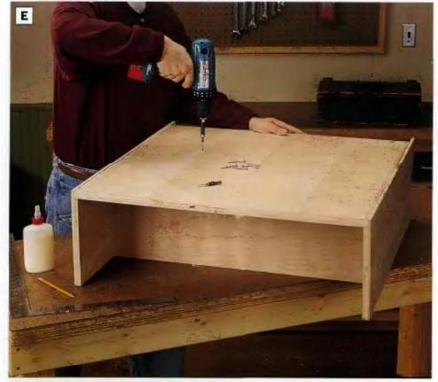
PHOTO E: Install the back on the bookcase with glue and screws driven into the back edges of the shelves. Mark the shelf locations on the back first, so you can drive the screws accurately.
