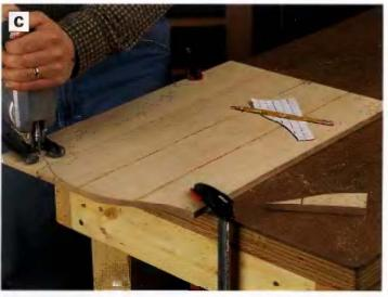
PHOTO C: Enlarge the Back Curve Layout grid pattern on page 237 to make a template for drawing the profile at the top of the back. Cut the profile to shape with a jlg saw.
