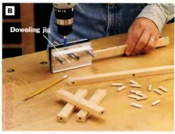
PHOTO B: Drill holes in the face frame ralls and sides so you can assemble these parts with dowels. A doweling jig ensures that the holes are positioned precisely across each joint and keeps the drill bit straight in relation to the workpiece.
