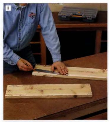
PHOTO I: Lay out the arm shapes on a pair of  $1 \times 6$  cedar boards.
