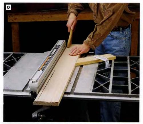
PHOTO 0: After the molding profile has been routed Into the edge of a wide, ¾-In.-thick oak board, rip-cut a ¾-In.-wide strip of the molding on the table saw. Repeat the process to make up as much molding as you'll need (about 13 lineal feet for the project as shown). This process is easier and safer than ripping the molding to width first and trying to feed narrow strips across a large cutter on the router table.
