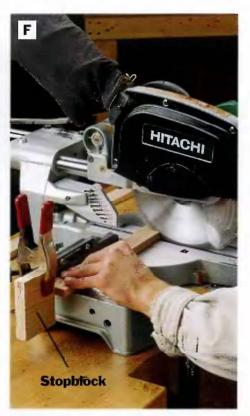
PHOTO F: Clamp a stopblock to the fence of a power miter saw, 11 in. from the edge of the blade, to make uniform cross-cuts when cutting the rails and handle pieces to length.
