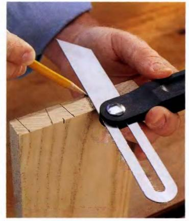
After edge-gluing and cutting the workpieces to size, begin work by laying out the pins. Use the drawing labeled "Pin/tall layout" to lay out the pins on the end of the board with a pencil and the adjustable square.
