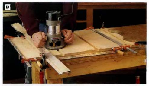
PHOTO B: Clamp the sides together side by side, lay out the shelf dado locations and gangrout the dadoes across both sides. Clamp a straightedge across the side workpleces to guide the router cuts.
