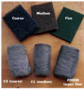
STEEL WOOL AND ABRASIVE PADS (synthetic steel wool) have many uses in the shop, from general cleanup to buffing to stripping old finishes.
