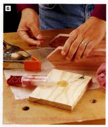
PHOTO G: Spread two-part epoxy Into the grooves in the side panels, remove the protective film from the PlexIglas end pieces, and slide the end pieces Into the grooves. The end pieces should stop 34 in. from the bottoms of the sides.
