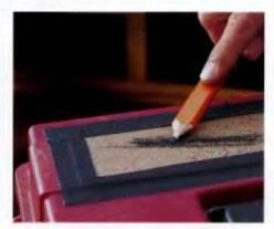
ATTACH MEDIUM-GRIT SANDPAPER to your toolbox to make a convenient and safe sharpener for lumber penciis.
