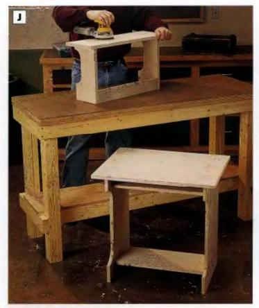
PHOTO J: Once you've filied all the screwholes and any voids in the plywood, sand the bench and desk before you prime and paint. A randomorbit sander and 150-grit sandpaper will make this a quick task.
