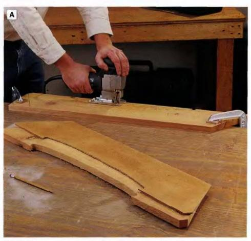
PHOTO A: Lay out and cut a template for making the sides of the ralling planter, then use this template to draw the shapes on the side workpieces. Cut out the shapes with a jig saw.
