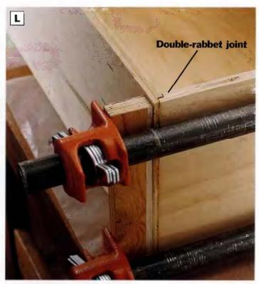
PHOTO L: The glued double-rabbet joints used to construct the drawer boxes are strong enough that no additional reinforcement is needed. Do not use glue or fasteners to secure the drawer bottom, which is inserted into the inside grooves prior to drawer assembly.
