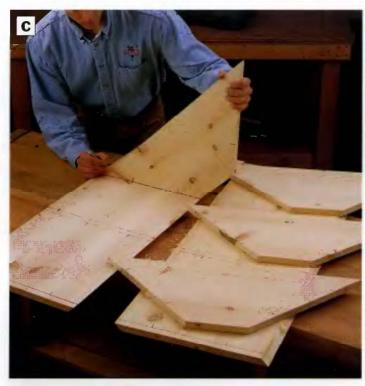
PHOTO C: Lay out all the carcase parts and draw alignment marks for biscult joints. Be sure to keep the orientation of the side panel bevels in mind when you lay out and mark the parts.
