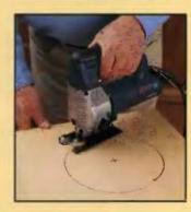
KEEP PRESSURE DIRECTLY ABOVE THE BLADE, Whether you're using a top-handle saw, like the one above, or a barrel grip saw, hold the tool so your hand is forward and directly above the blade area. Take care not to force the saw: the blade will break or deflect from the cut Ilne.
