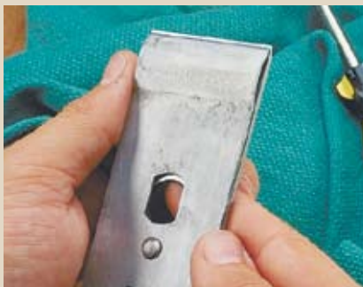
2 After smoothing the edge of the cap iron, tighten it in place behind the leading edge of the blade.
