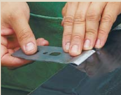
1 Lower the back end of the cap iron slightly, then sand the front edge by making a few smooth strokes.
