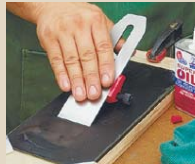
2 A honing guide ensures that the blade remains at a consistent angle as you're sharpening.
