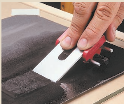
2 By holding the blade at a consistent angle, a honing guide ensures that the bevel stays flat.
