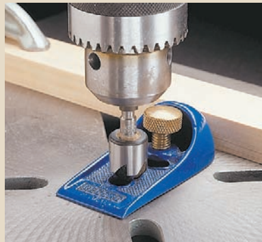
1 With the lever cap against a fence clamped to the drill press table, countersink the key-
