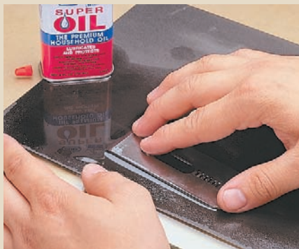
1 Using oil as a lubricant, you can sand the back of the blade with a piece of silicon carbide paper.
