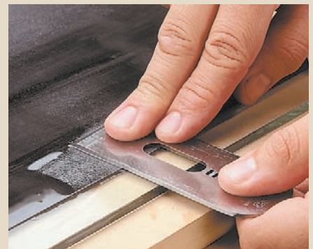
3 To remove a burr, alternately sand the bevel and the back with the final grit used to flatten the back.
