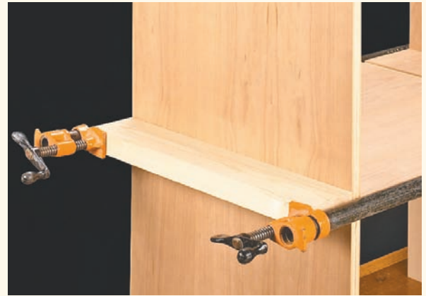
▲ The stout cauls used for this partial assembly are slightly bowed through the middle. This spreads the force of your clamps across the entire joint.
