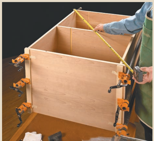
▲ Comparing opposite, corner-to-corner measurements is your best bet when checking a case for square. If the measurements are equal, you know the case is square.
