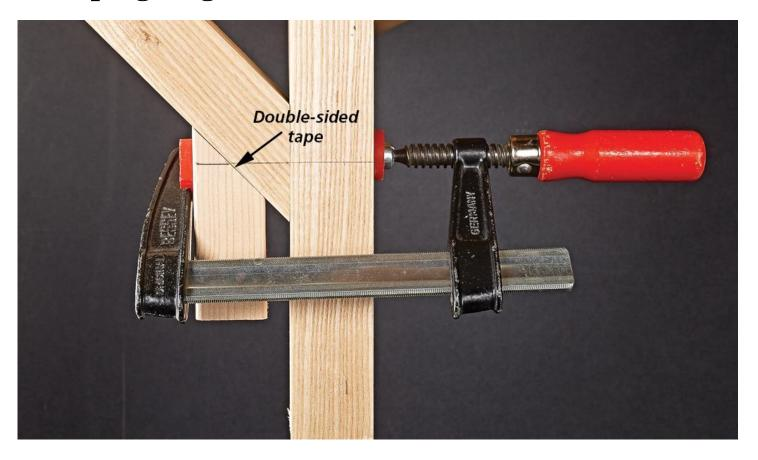
Bill Wells of Olympia, Washington, came up with a clever solution for gluing an angled piece to a flat surface without using fasteners. He simply uses the angled cutoff piece as a clamp block and some double-sided tape between the parts. A bar clamp holds everything together.
