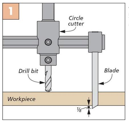
To do it, adjust the drill bit on the circle cutter so it's higher than the depth of the cutting blade by the thickness of the workpiece, plus 1/8", as shown here.
