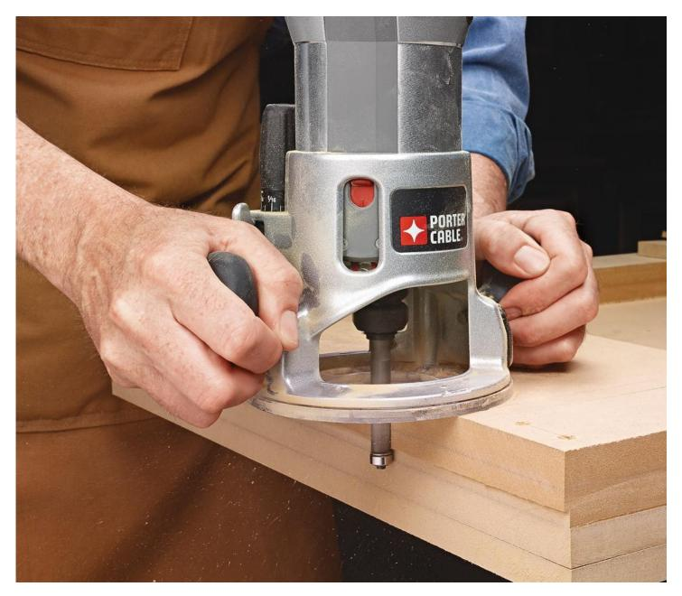
I recently made a new workbench for my shop. The top consisted of several layers of MDF. After gluing the MDF panels together, I was faced with the task of trimming the ends to length. The bench top was too big and heavy to run through the table saw. And it was too thick to make the cuts in one pass with a circular saw. Instead, I used this three-step process using my circular saw and router with a flush trim bit installed.
