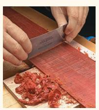
**Milling Marks.** Band saw marks from the sawmill are common. But a hand scraper will smooth them out.
