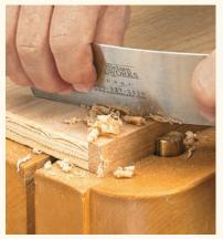
**Plywood Edging.** A scraper excels at leveling edging on plywood without damaging the veneer.
