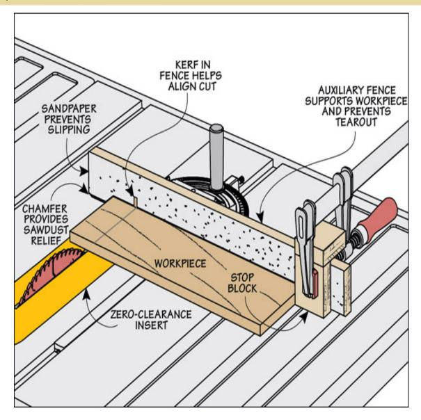
The first step is to add a long, auxiliary fence to the miter gauge. The fence I use is just a strip of plywood that extends beyond the blade to fully support the workpiece. Some self-adhesive sandpaper keeps the workpiece from shifting during the cut.
