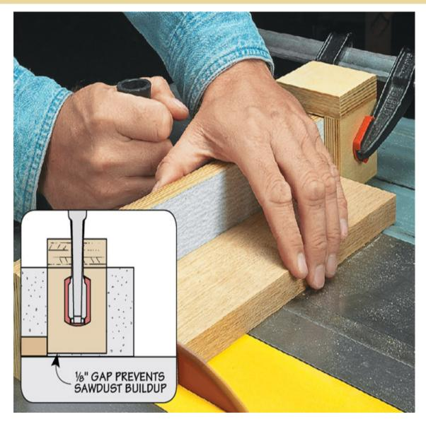
When I need to make several identical parts, I made an L-shaped stop block. Clamping the stop block to the fence guarantees parts are the same exact length. I sized the stop block so it's slightly shorter than the fence. This slight gap prevents saw dust building up against the block that could spoil the cut, as shown in the inset drawing.
