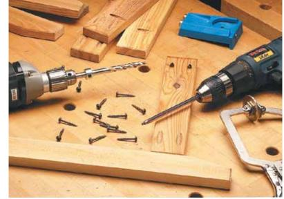
jigs available. But they all do exactly the same thing. They guide the drill bit so it will drill an accurate hole exactly 15° into the face of a workpiece, as shown in Figure 1. That's all there is to it. Note: The jig shown is made by *Kreg Tool Company*.
