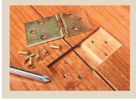
The short leaf of a table hinge is mortised into the top. The long leaf is mortised into the table leaf. You'll need to cut a narrow slot in the mortise to accommodate the barrel of the hinge.
