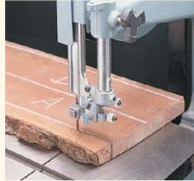
▲ **Roughing it.** Cutting pieces to rough size first means there's less material to remove to get them flat and straight.
