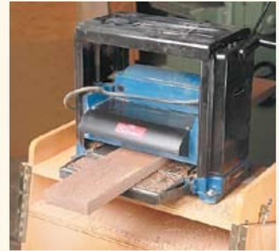
▲ **Thicknessing the stock.** A planer not only reduces the thickness of the board, it creates a face that's flat and parallel to the jointed face.
