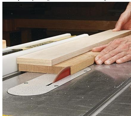
For many of my woodworking projects, I use short pieces of rough-sawn stock. Some of the edges are too uneven to safely run them through my jointer to true one edge. Instead, I devised the following technique that allows me to cut one straight edge using my table saw. Start by placing the rough-sawn piece against the rip fence. Position the fence to get the best use out of the board and lock it down.
