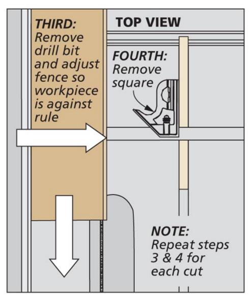
Now I can remove the drill bit and adjust the rip fence until the workpiece touches the end of my rule. Then just remove the square and make the cut.
