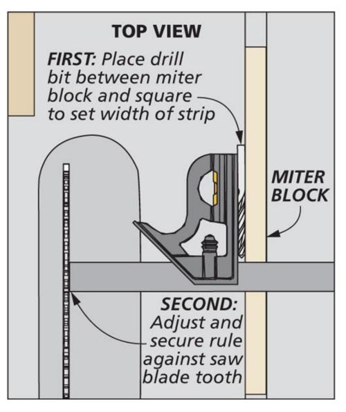
Start by cutting a block that fits snugly in the miter slot and sits proud of the saw table by <sup>1/4</sup>'. Using a drill bit as a spacer to set the thickness of the strip, I adjust my combination square so that it just touches a tooth on my saw blade.
