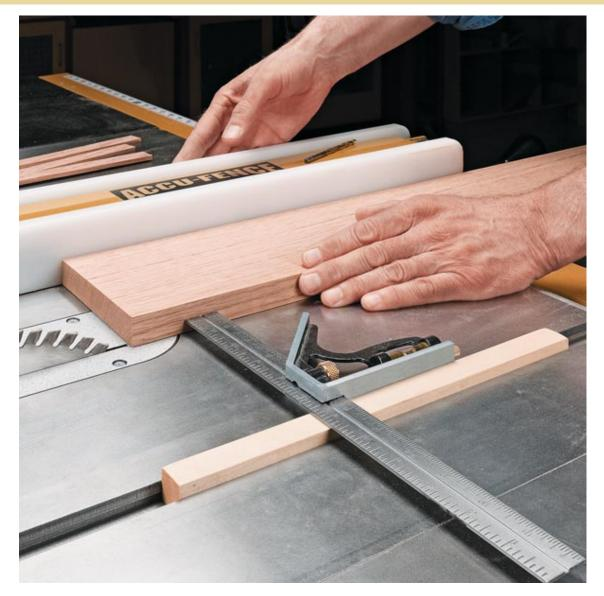
When making plywood shelves, I like to cover the front edge of the shelf with a thin strip of hardwood. Making the strips can be a challenge, though. If the strips are cut between the blade and rip fence, there's a chance the small piece will kick back. But cutting the strip on the left side of the blade requires adjusting the fence between each cut, introducing possible error.
