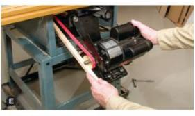
Eliminate vibration and you'll produce improvements at the cutting edge. Align your saw's pulleys and install a Power Twist Link Belt for smooth running.
