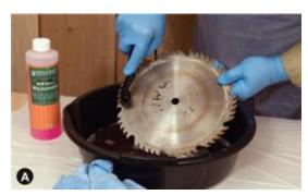
Before you ship the blade off to the sharpening shop, inspect it for a buildup of pitch and resin. You may discover that you have still-sharp teeth hiding under a layer of baked-on residue. Resin Remover, shown in Photo A, is a nontoxic concentrate that you dilute with water and apply by immersing the blade. Save and re-use the cleaning solution until it loses its effectiveness. After you've cleaned, water-rinsed, and air-dried the blade, give it a shot of Dri-Cote
