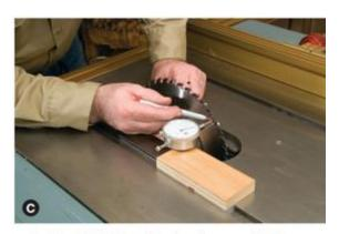
Check the blade's distance from the miter-gauge slot at two positions to make certain that it's parallel.
