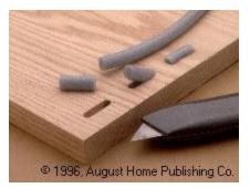
Recently I was working on a project that had a series of slats that fit in mortises. Because of the way the project was designed, it was easier to apply the finish before assembling all the pieces. The trick was keeping the finish out of the mortises — I wanted good glue joints later on.
