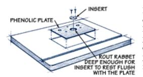
Replace your current insert, or make a new one from scratch. Buy a piece of plastic or hardboard, no more than half the thickness of your phenolic plate. Rout a rabbet into the current hole in your plate. Trace the outline of your insert on the plate, then bandsaw the new insert to size, and screw it in.
