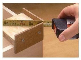
Comparing the diagonals of a cabinet or a box is a great way to check it for square. But when you're working alone in the shop, measuing long diagonals accurately can be difficult. To make this job easier, I made a pair of simple tape holders.
