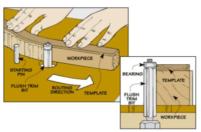
you can cut a full-size pattern out of paper and glue it to the hardboard. Then cut out the shape slightly oversize, and file (or sand) carefully up to the line.
