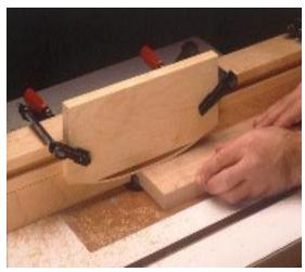
In use, the hold-down is clamped to the fence so enough downward pressure can be applied to the workpiece to keep it flat against the table top — without causing the workpiece to bind.
