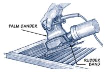
Hold the stick against the pad of your palm sander. Next, place a size 84 rubber band (available at office supply stores) onto the handle indentation of the stick and pull the rubber band up and over the edges of your sander. Hook it onto the other end of the stick. When you turn on your sander, the stir stick acts as a thin extension and fits perfectly between the louvered slats and into the corners, eliminating hours of tedious hand sanding.
