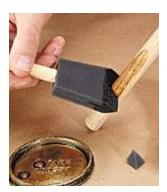
To provide better coverage when applying stain to a dowel, *R*. *B. Himes of Vienna, Ohio* cuts a V-shaped notch in a foam brush.
