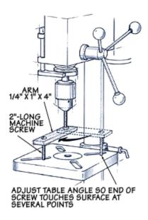
I have a small bench top drill press with a table that tilts to accommodate drilling angled holes, which is very handy. Unfortunately, it doesn't have any stops or markings to let me know when I've got the table set back square to the spindle and bit.
