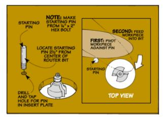
To reduce the chance of that happening, I use a starting pin. This is just a cutoff bolt that threads into a hole in the insert plate.
