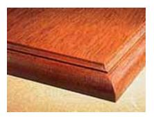
When applying liquid stains, the stain soaks more deeply into the pores of the end grain than the face grain, darkening the ends much more than the faces, see top photo.
