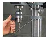
I'm always misplacing the chuck key to my drill press. So I fastened it to a retractable key chain that's attached to the column of the drill press, see photo.
