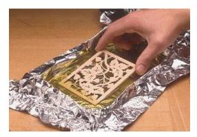
As for applying a finish, we get into the tiny openings by dipping the panel in an oil finish, see photo at right. When dipping a fretwork panel, aluminum foil shaped into a tray acts as a reservoir for the oil finish. To remove the excess finish, you can blot the panel dry with a cloth or blow it out with compressed air.
