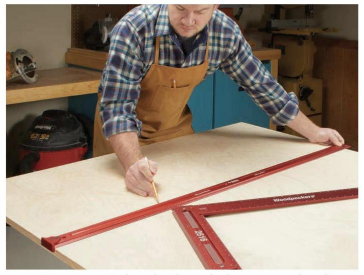
**Accurate Layout.** No matter how talented a woodworker you are, your layout lines are only as accurate as your layout tools. Investing in a high-quality set of accurate layout tools for large plywood sheets will help the entire building process go much more smoothly.
