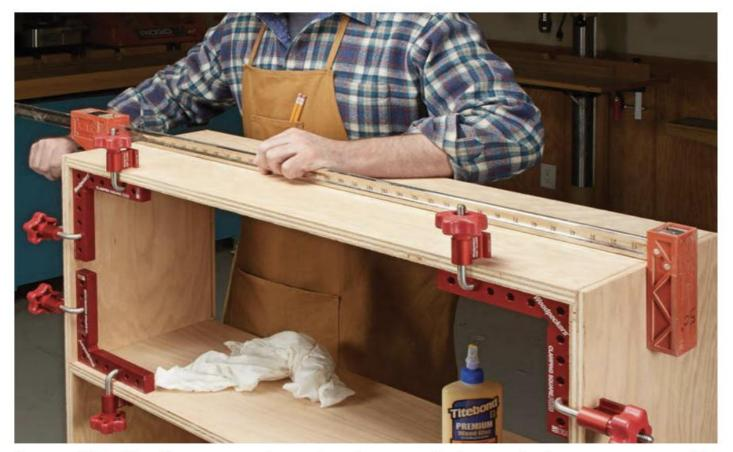
**Square Glue Up.** Once corner clamps have been applied guaranteeing a square assembly, you can work around the case adding additional clamps. I'll often leave the clamps in place until the glue is dry, even if there are screws holding everything together.
