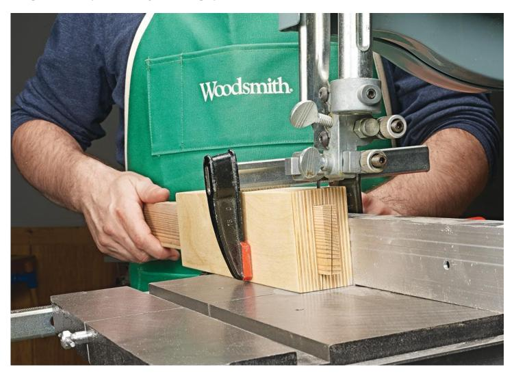
Building dollhouses is one of my favorite woodworking projects. But I was never quite comfortable making the clapboard siding on the table saw. The small, thin pieces that I needed to bevel rip for the siding blanks put my fingers too close to the spinning blade. To solve this problem, I designed this simple jig to use on my band saw.
