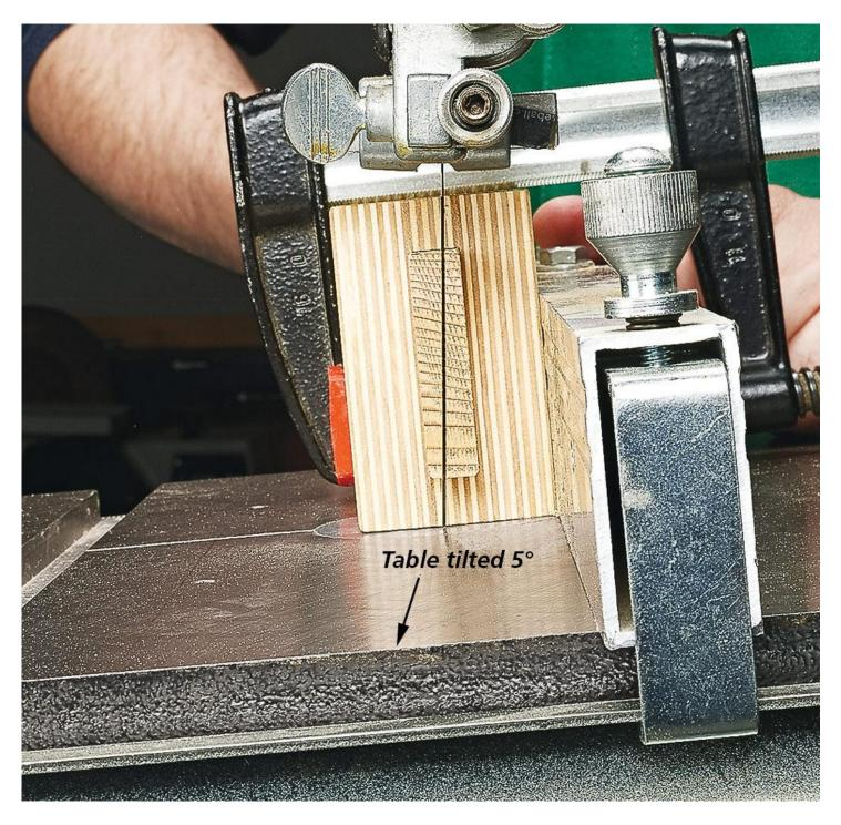
The setup couldn't be easier. Just tilt the band saw table to  $5^{\circ}$  and set the fence so the jig is positioned as shown in the inset photo above. Cut into the jig about 1/2" and clamp the jig to the fence. Now feed the blanks through the jig. Use another blank as a push stick to move the workpiece through the jig.
