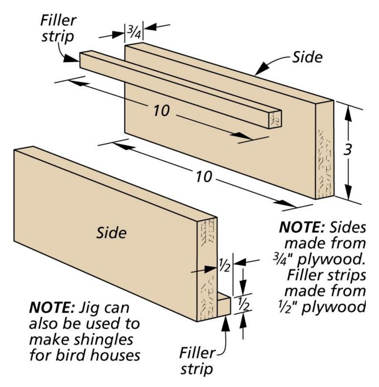
The jig is simply two plywood sides with a couple plywood filler strips glued to the inside face of each side. The opening created between the filler strips is sized to accommodate a rectangular blank that will yield two tapered siding "strips" when ripped in half.
