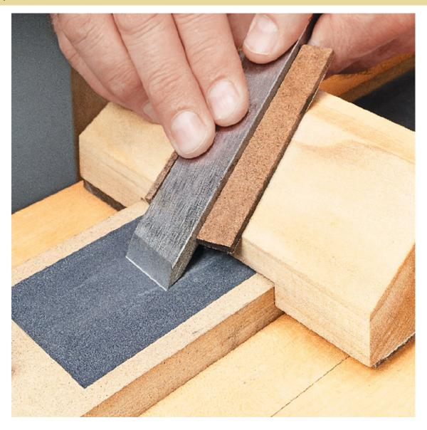
I have a couple of tools with skewed blades. I find it a difficult task to sharpen these tools with a standard honing jig. So I built the jig you see here. This jig holds the blade at the proper angle to the sharpening surface so I can hone a perfect edge identically every time I use it.
