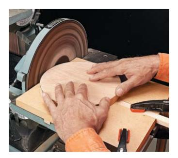
Creating perfect circles on a disk sander is a snap with this simple jig. Basically, the jig consist of four parts: an MDF base, a cleat, an adjustable hardwood runner, and a pivot pin made from a dowel, see drawing at right.
