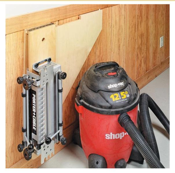
The platform is attached to the wall bracket with a hinge block and continuous hinge. The folding support is also attached to the bracket with a hinge.
