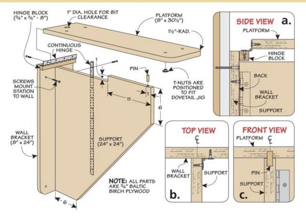
As you can see in the drawings, the station consists of three basic plywood parts: a wall bracket, a folding support, and the jig platform.
