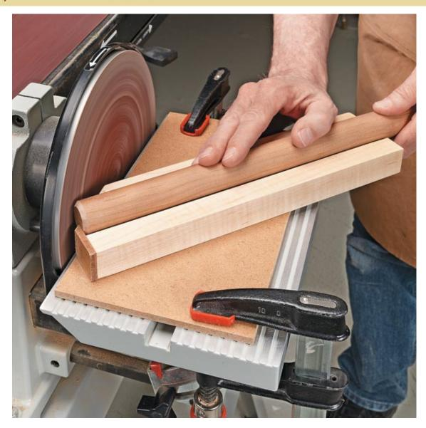
I use dowels in a number of projects around my shop. For a clean appearance, and to soften the sharp edges, I like to chamfer their ends.
