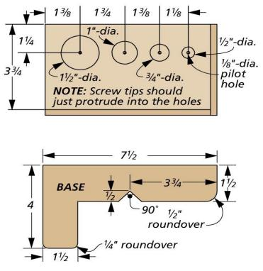
One note about constructing the center-finding block: drill the four shallow holes using Forstner bits. The tip of the Forstner bit leaves a small divot in the bottom of each hole. Use this divot to drill the through holes. The tips of the 1" screws should just protrude into the holes.
