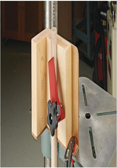
It seemed like no matter how well I marked the centers of dowel ends, I could never get a perfectly centered hole. That all changed when I came up with the jig you see.
