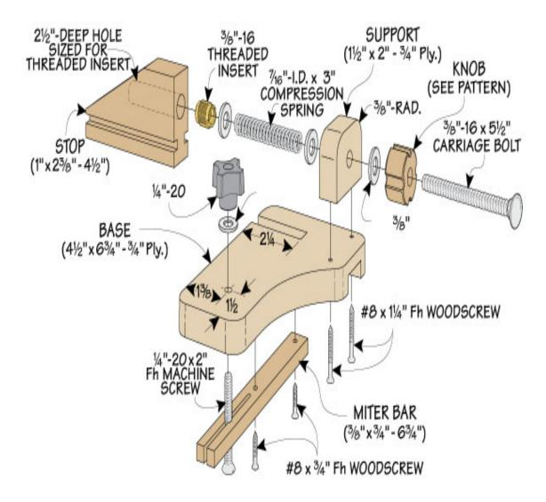
The drawings in this tip show how to make all the pieces, starting with the base. A tapered stop slides along a slot in the base controlled by a shop-made knob and carriage bolt. The spring supplies constant pressure on the workpiece.
