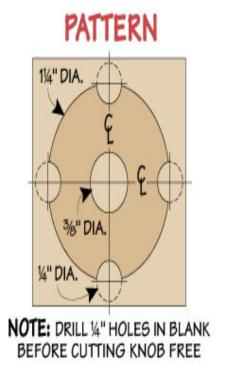
A knob can be made by drilling 4 holes in a piece of plywood before cutting it free, shown in the pattern. Each complete turn of the knob moves the stop 1/16".
