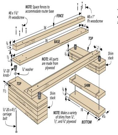
The leveling jig is nothing more than two router guides consisting of a base and a fence. The router guides are attached at either end to a couple of shim stacks.
