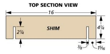
The shim stacks have a solid top and bottom, but the shims in the middle of the stacks are slotted to allow them to be easily added or removed (detail 'a'). The leveling jig is set in position over the workpiece. I place an equal number of shims in each shim stack until the router guides just clear the highest point of my workpiece. The four knobs are then tightened down.
