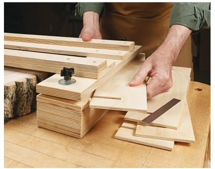
To use the leveling jig, you'll need to place it, and the material being leveled, on a flat surface. My workbench works fine for this. If your material isn't heavy enough to stay in position, you may need to use a non-slip pad to keep it from sliding on the workbench.
