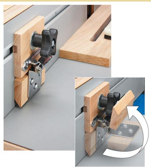
A flip-up stop block is a great addition to any router table or table saw miter fence. The bottom block just flips up out of the way when not in use.
