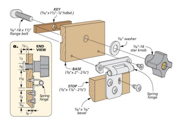
I used a spring hinge to keep the block raised when it's not in use. As you can see in the drawing, the spring hinge is attached to the face of each piece. The top piece holds the flange bolt and knob that keep the block in place in the fence track. I cut a bevel in the bottom block to help prevent sawdust build-up.
