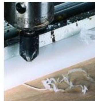
Use a fence on your drill press's table when drilling the holes and countersinks in the miter bar. Though I'm sure some of us could freehand this operation, a fence ensures your success.
