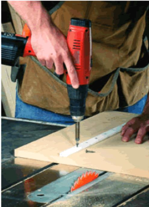
The number of screws looks like overkill, but they help prevent the bar from flexing and they allow you to take out any side-to-side play in the plastic bar by tightening the screws slightly
