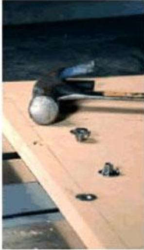
T-nuts are easy to install using a hammer if you drilled your holes correctly in your base. Drill the  $\frac{3}{4}$ "-diameter hole for the flange using a Forstner bit. Then use the hole left by the bit's spur to center the  $\frac{5}{16}$ " bit for the through-hole.
