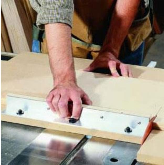
don't find on most people's sleds: First, you can square it to the blade and recalibrate it when necessary (such as when you drop the jig or your saw's settings change). Most sleds don't have this feature and need to be trashed when they eventually become inaccurate.
