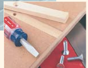
▲ Ripping. To rip a straight edge on a rough board, just remove the runner and use the rip fence to guide the jig.
