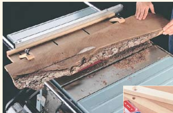
▲ Ripping. To rip a straight edge on a rough board, just remove the runner and use the rip fence to guide the jig.
