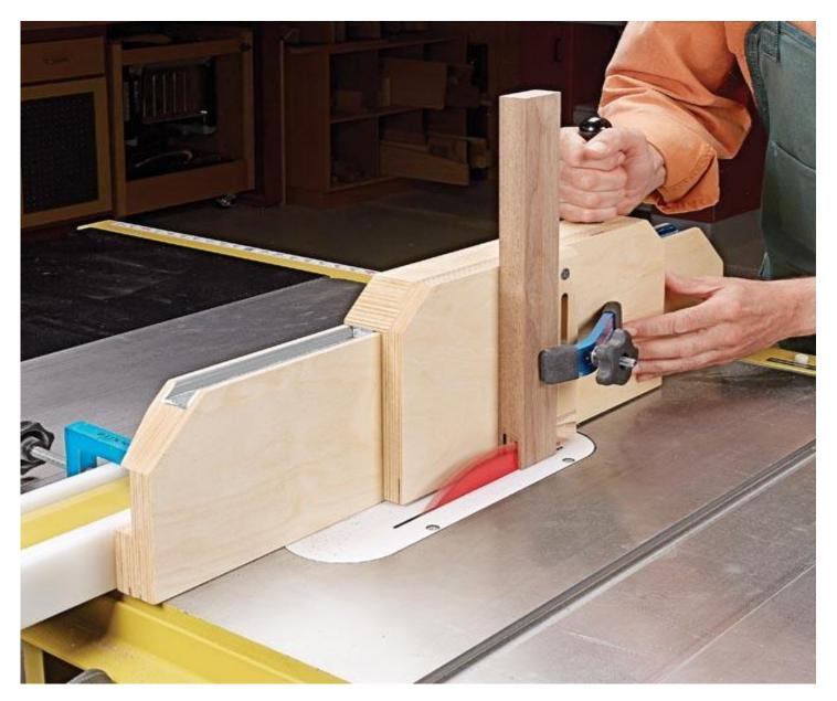
The jig just requires a few parts and hardware, and it's easy to make, as shown below. It consists of two basic components: a fence and a guide. The fence mounts to the saw's rip fence with two commercial fence clamps. This makes it easy to adjust the fence in relation to the blade. On its own, the fence is a great tall auxiliary fence.
