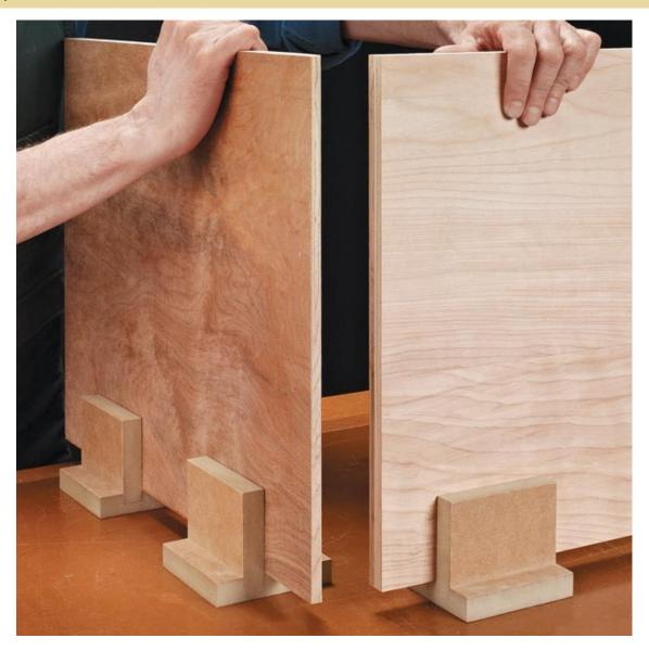
The key to a solid case is getting all of the pieces square. But trying to balance wide workpieces on edge during assembly can really be a challenge. The stands you see here are the perfect solution. The simple design makes it easy to stand your workpieces on edge.
