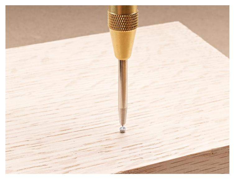
Instead of putting larger holes in trim work using a nail set, *David Fraser* of Modjeska Canyon, California sets the nail heads with an automatic center punch.
