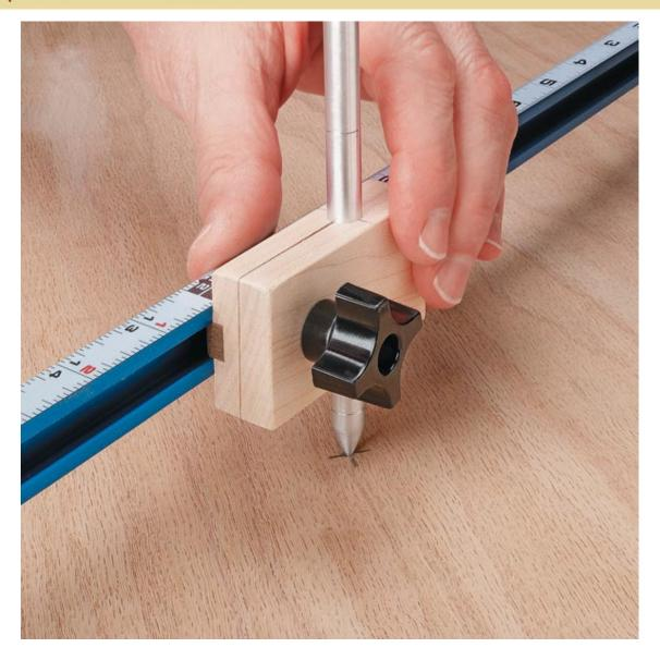
The trammel heads are made from hardwood. The vertical holes are sized to fit a pencil and aluminum rod. To sharpen the rod, just chuck it in the drill press and file it to a point. A through hole accommodates the flange bolt that secures the head to the T-track.
