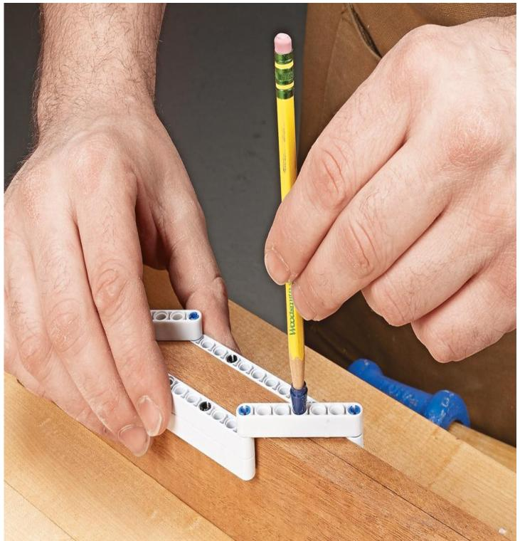
William Collett of Bettendorf, Iowa, found a clever way to make a center-finder tool using some of his child's toys. He simply connected Lego pieces like the ones shown above. With a pencil in one end piece, the center-finder adjusts for varying thicknesses of lumber.
