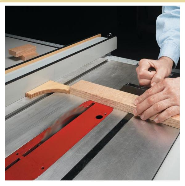
It's a tricky task to crosscut short, identical pieces. Here's a safe, easy solution. The way it works is that a magnetic stand-off block is butted against the rip fence in front of the blade. The block acts as a length stop while leaving plenty of clearance to avoid any chance of kickback.
