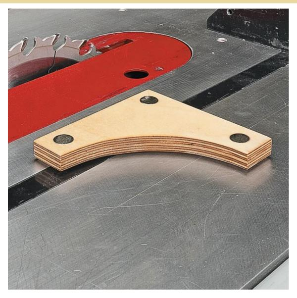
The stop is made from a scrap of plywood. A few rare-earth magnets are installed in counterbores on the bottom face.
