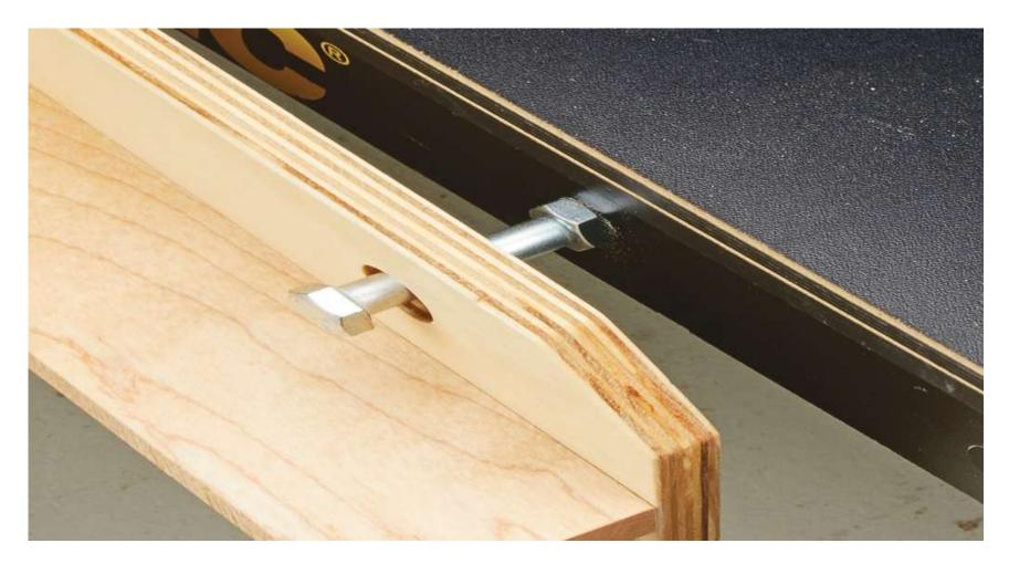
A pair of oversized holes in the crosscut sled easily slip over the bolt head, yet still hold it secure. **Short Wing.** The solution came in the form of the wing on my table saw. The wing is shorter than the fence rail, and allowed enough room for me to hang the sled.
