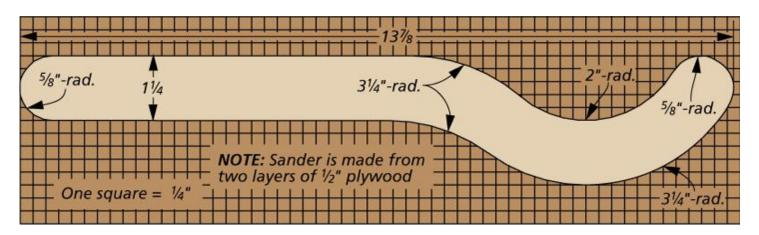
I size my detail sanders for use with 1 x 30 sanding belts but other sizes will also work. The important thing to remember is the shape of the sander. They are designed so that when gripped near the curved end, the belt is properly tensioned to stay in place. I usually cut them a little oversized and sand them down to fit.
