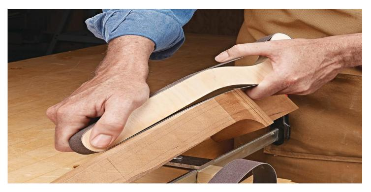
Sanding curved parts with power sanding equipment can be nearly impossible. Instead, I like to turn to hand sanding for smoothing these parts. To aid in sanding these curvy pieces, I always keep one of these shop-made detail sanders on hand.
