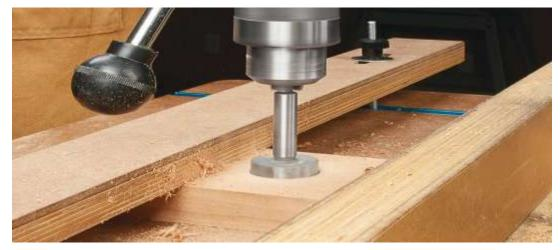
Using it is just as simple as the construction. After positioning my workpiece, I can place the bar on top and clamp it down using the knobs. That way, the workpiece is held secure and my hands are out of the way.
