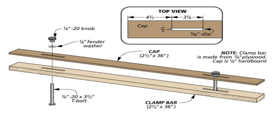
**Clamp Bar.** As you can see in the photo, the hold-down is nothing more than a long piece of plywood with a hardboard cap glued on it. A slot in each end lines up with my T-track and is the attachment point to my drill press table.
