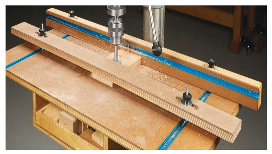
If you're anything like me, holding parts at the drill press tends to be hard on your hands. After having a piece grab and spin around, I decided to make the simple clamping jig shown here.
