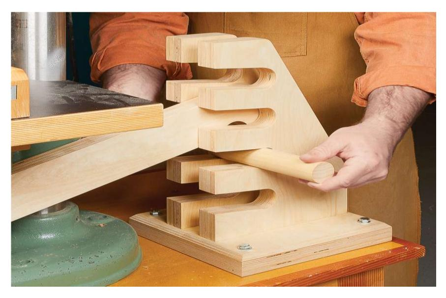
By moving the dowel up or down in the uprights, the jack can cover a range of height adjustments.
