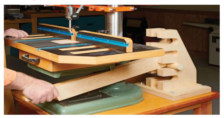
My drill press doesn't have a crank to raise and lower the table. So moving the table on my drill press can be a pain. Not only is it heavy, but it's hard to get a good grip to both lift and lock it in place. I decided to tackle this problem by building the jack shown above.
