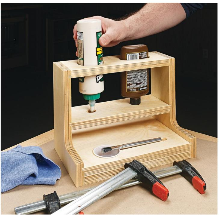
Waiting for glue to flow from the bottom of the glue bottle to the tip is one of my pet peeves in the shop. Instead of waiting, I store a couple bottles in this handy rack that keeps the bottles upside-down so the glue is always ready to go.
