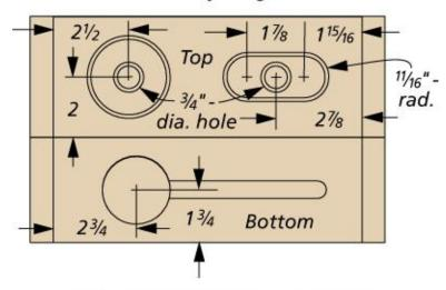
NOTE: Chamfer edge of holes 1/8"
