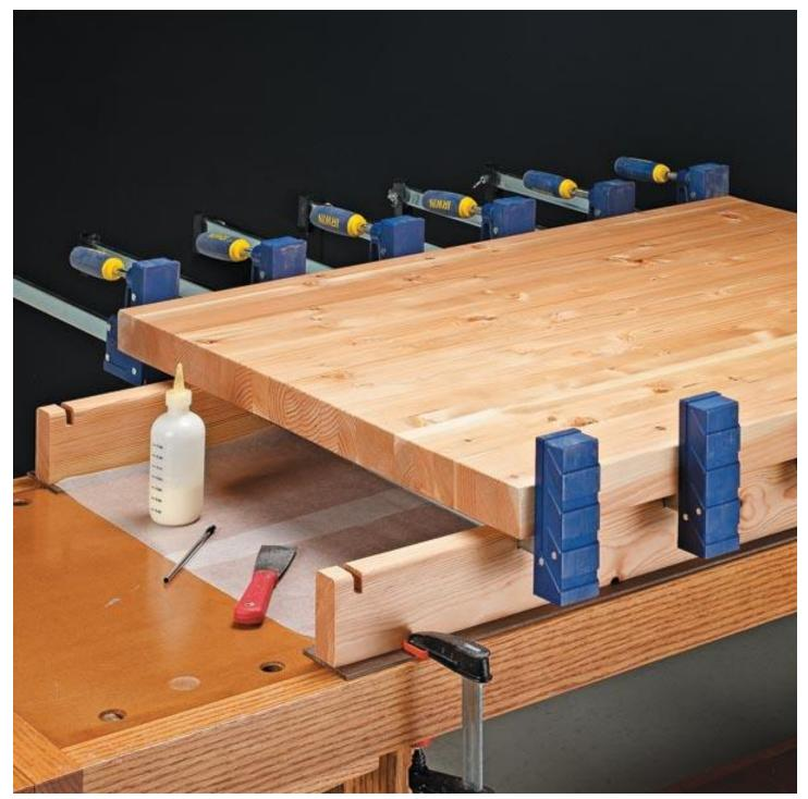
Gluing up wide panels can be a chore. This is especially true if the panel is wider than your workbench because it's almost impossible to stand the clamps up while positioning your workpieces. To avoid this hassle, I came up with the solution you see here.
