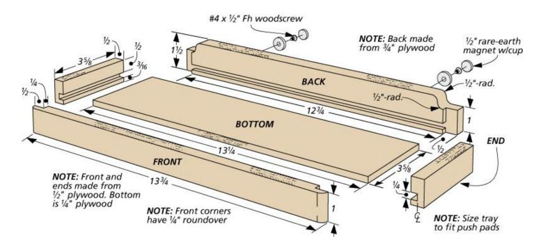
As shown here, the push pad tray is constructed from plywood. The front, back, and end pieces all have a groove along their inside edge. This groove holds the plywood bottom panel. The back and front pieces also receive a rabbet along their ends. These rabbets interlock with the end pieces to make a sturdy tray.
