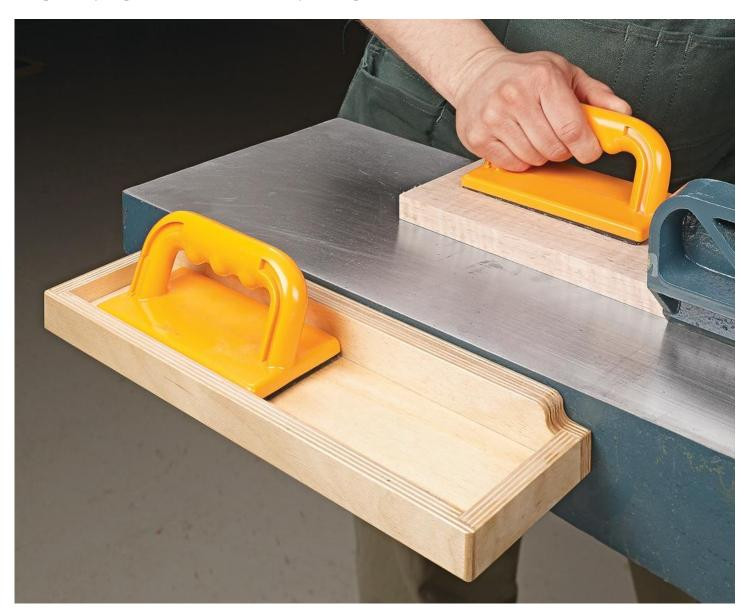
A good set of push pads is a must-have safety item when using a jointer. And the jointer bed seems like the logical place to store them. That is until you walk over to your jointer, with board in hand, and realize that the push pads are right in the way of where you need to set the workpiece. Well, this handy, easy-to-mount tray solves that problem while keeping the push pads at the ready.
