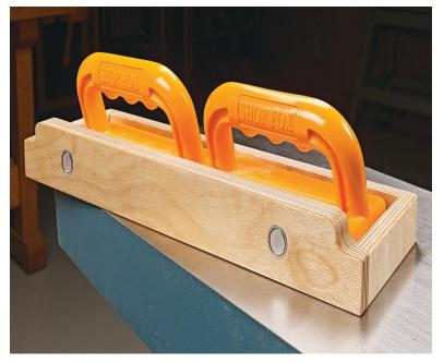
I also rounded over the ends of the front piece to keep from snagging my shop apron. I drilled a couple shallow holes in the back of the tray to recess two rareearth magnets and cups. These are more than enough to hold the tray to the jointer. The tray then goes together with a little glue at the corners and in the groove.
