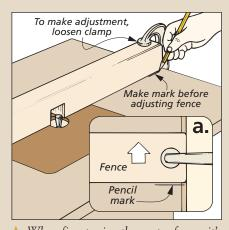
When fine-tuning the router fence, it's hard to see how much it's actually being moved. So to make the adjustments easy to see, I simply make a reference mark beside the fence.
