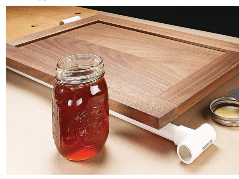
To support a workpiece while gluing or finishing, Dave Youngren of Clovis, California, uses ¾ PVC pipe with a tee fitting on the ends to keep the pipe from rolling. The supports are inexpensive to make and can be easily cleaned off when they get too messy.
