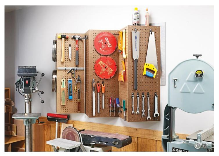
One day while working at my bench, it occurred to me that I could gain additional storage space on my pegboard rack without increasing the size of the footprint on the wall. To do this, I made the panels into three-dimensional sections, as shown in the photo above.
