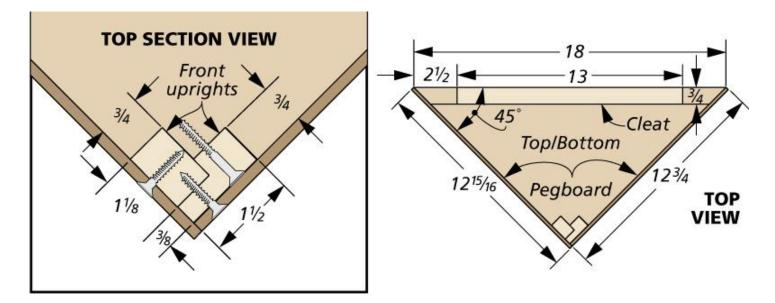
Each section consists of a triangular frame with two pieces of pegboard attached to the front face of each frame. A pair of cleats on the back of the frame provides a surface for mounting each section to the wall. And the top and bottom panels, along with the uprights, add rigidity to the assembly. The top panel even doubles as a small shelf.
