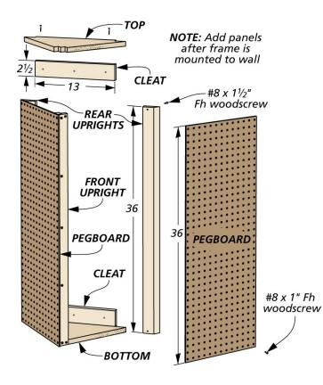
I mounted the frames to the wall through the cleats before screwing the pegboard sections to the frame. This configuration as shown added over 40% more surface area.
