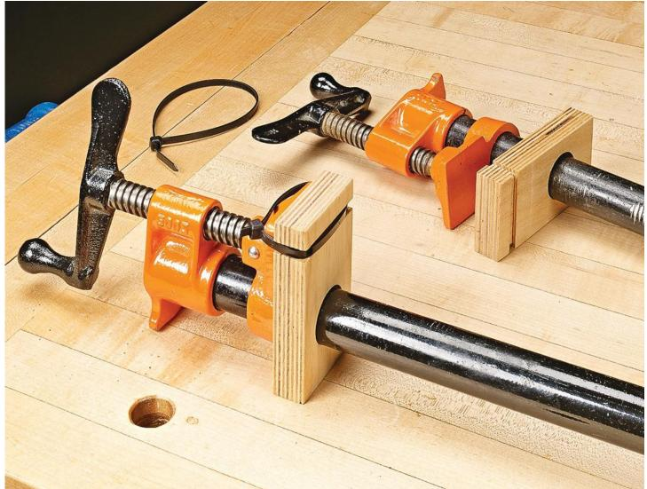
Denis Manigart of Ampang Jaya, Malaysia, couldn't justify the expense of buying clamp pads for all of his pipe clamps. Instead, he made some out of plywood. Each pad has a hole for the pipe to fit through and a groove to secure it to the clamp with a cable tie.
