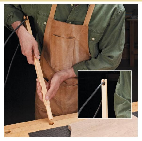
You start with a long piece of wood and cut a slot on one end to hold the cord up and out of the way. Then round the edges of the square board on your router table so it will fit neatly in a dog hole on your bench. Now your cords are contained and never in the way.
