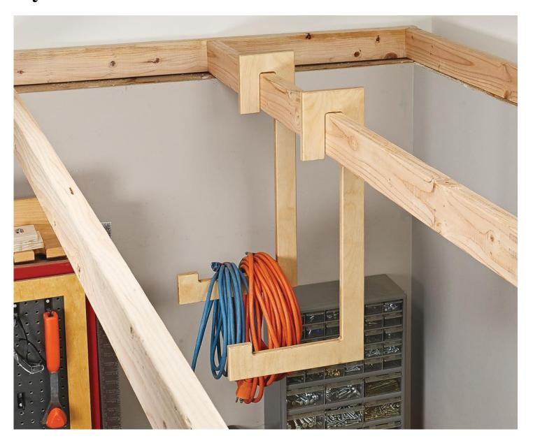
Needing a quick and customizable storage solution for hanging extension cords and other lightweight items, Lyle Qualley of Tekamah, Nebraska, made a couple simple rafter hooks from leftover plywood. The hooks are made to slip over the exposed rafters in his shop. He sized his hooks so they were easy to reach without a stool, yet high enough to be out of the way.
