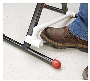
By using a  $90^{\circ}$  street elbow above the snap tee the brace can easily be disengaged by slipping your foot underneath the pipe and popping the snap tee off the leg of the roller stand.
