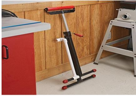
The support brace conveniently folds up alongside the roller stand, allowing the entire unit to be stored together.
