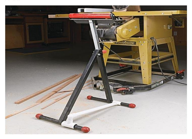
Some shop roller stands tend to fold up easily when using them. This can be especially dangerous if the stand is being used for outfeed support while cutting material at the table saw. I solved this problem by making a brace out of PVC pipe. The brace slips over one leg of the support stand and snaps down over the other when the stand is open to lock the legs apart. When you want to fold up the stand, the brace folds up, as well!
