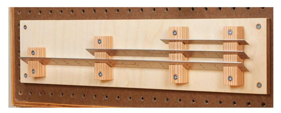
The different depth kerfs in the ribs allow plenty of room to remove even the smallest rule.
