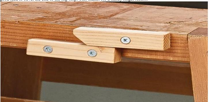
There are a couple of things to keep in mind when locating the flip stop. First, when it's in the down position, it must be below the top of the <u>sawhorse</u> (photo above). This way, it won't be in the way when you're not using it.
