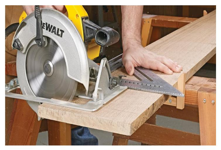
One of the cardinal rules of using a <u>circular saw</u> is to make sure your board is secure before making a cut. But to be honest, I don't always follow that rule. So instead of concentrating on the cut, I end up trying to keep the board from sliding across the sawhorse. To solve this problem, I installed two flip stops on each of my <u>sawhorses</u>.
